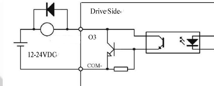
**Figure 3.4: Output Interface Wiring**
