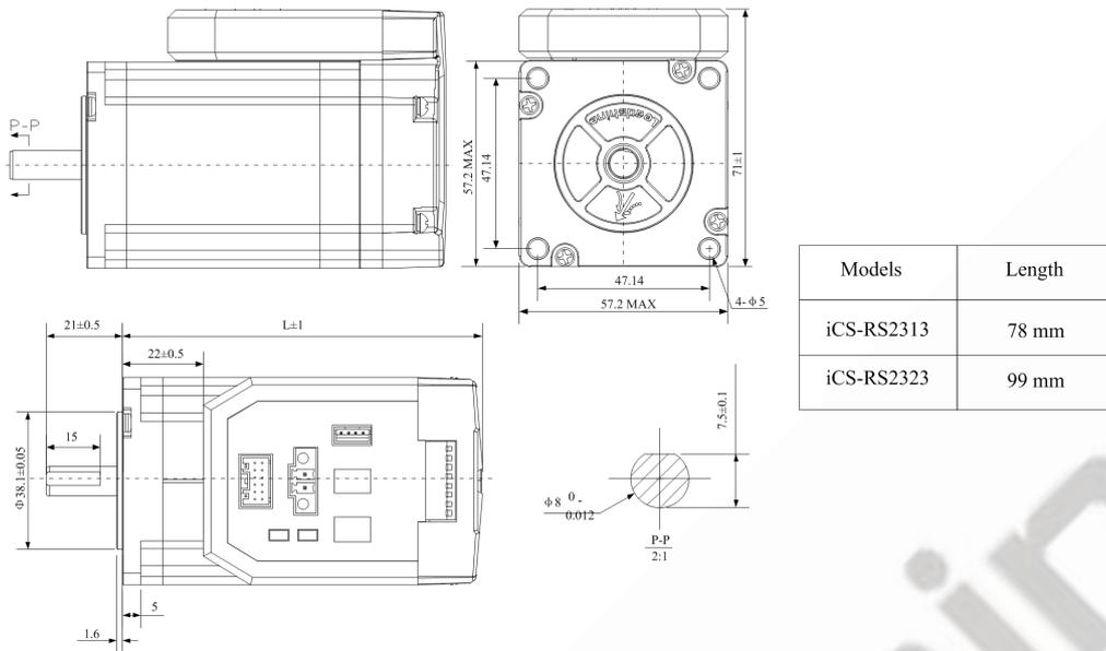
**Figure 1: Mechanical specifications**
