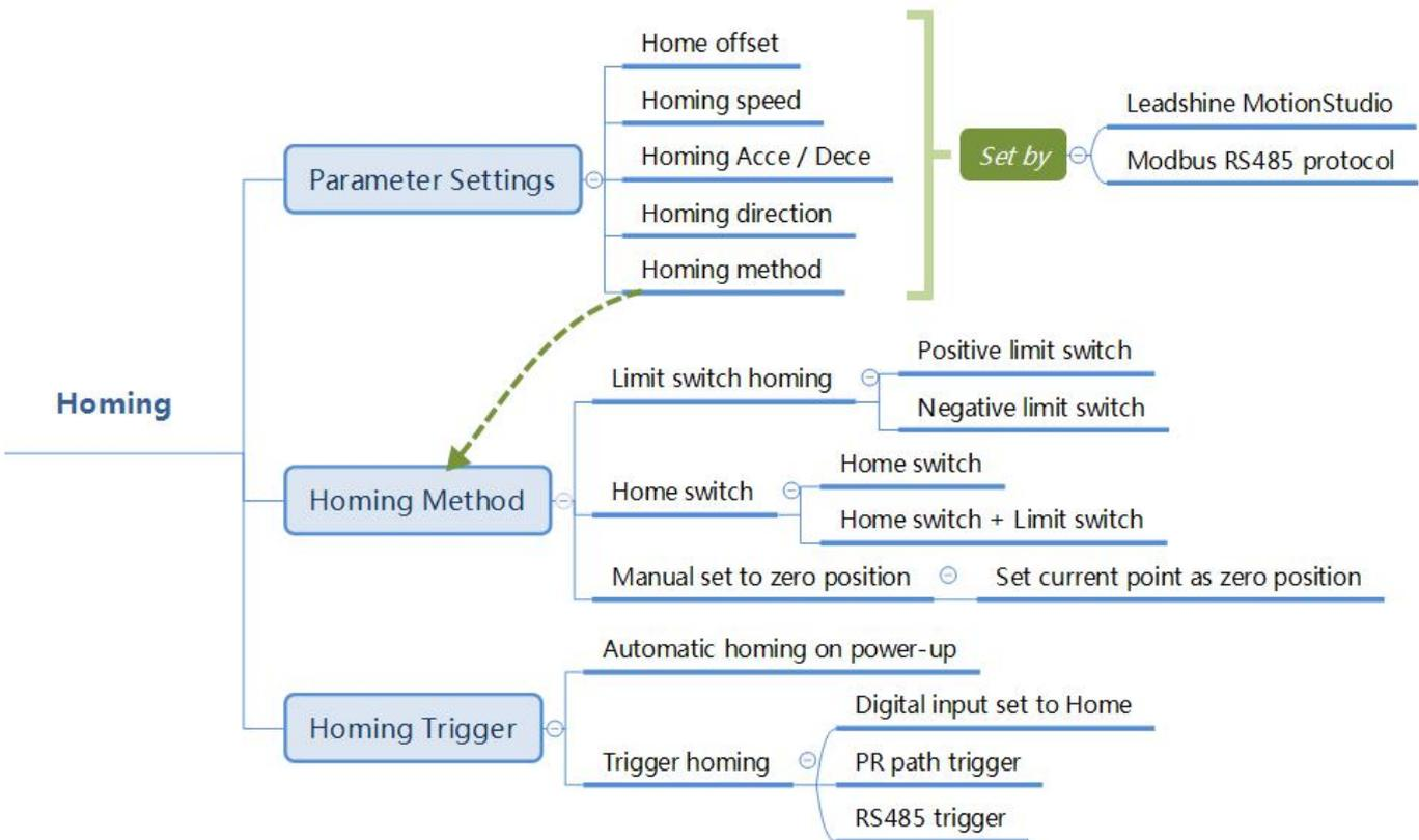
**Zero Position:** a fixed position on the machine can correspond to a definite digital input signal, or to a Z signal
