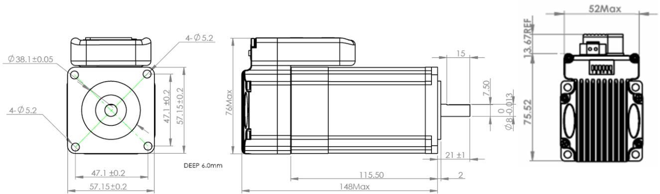
Mechanical Specification of iSV-B23180T-D4
