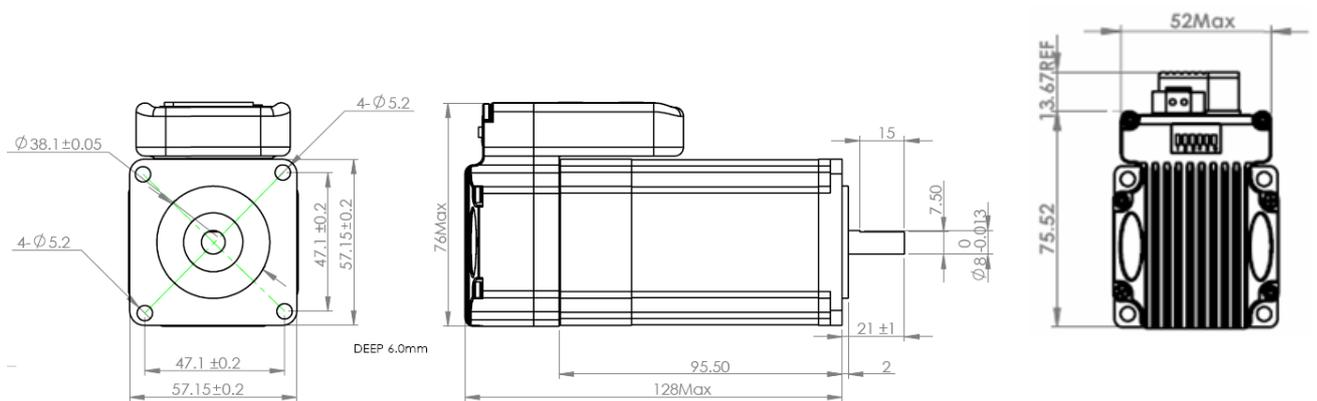
Mechanical Specification of iSV-B23130T-D4
