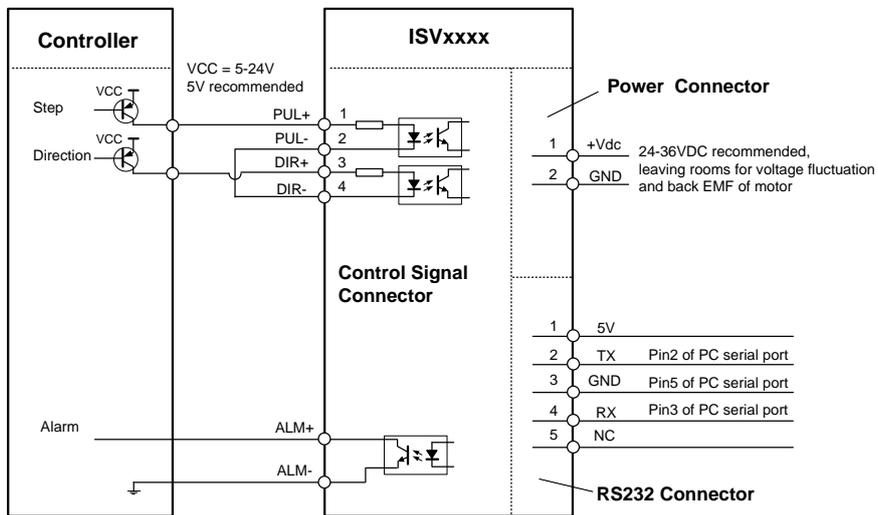
Connect iSV-Bxxx to controller of sourcing output
