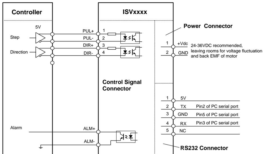
Connect iSV-Bxxx to controller of differential output
