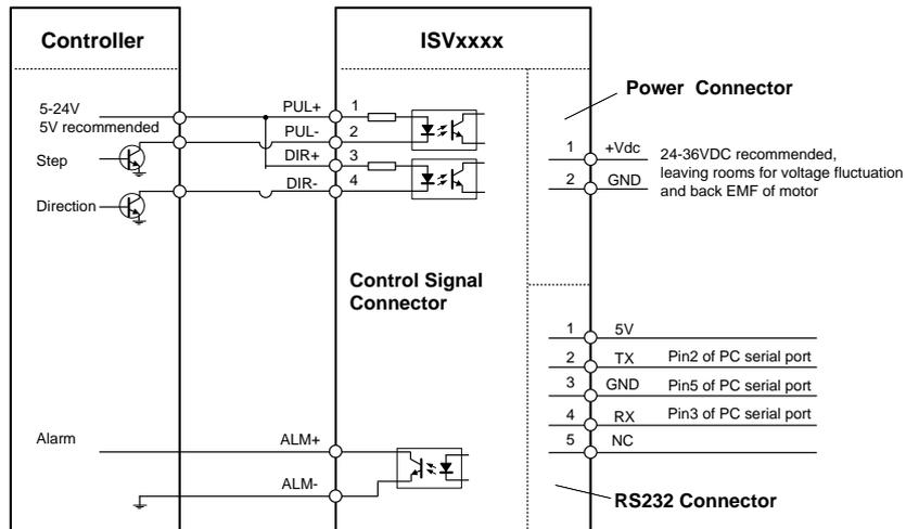
Connect iSV-Bxxx to controller of sinking output
