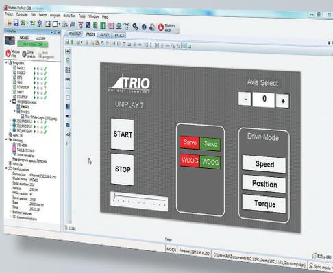
No additional software is required; UNIPLAY HMI's work with the Trio MC4+ *Motion Coordinator* range. *Motion Perfect* v4 is used to create operator HMI screens which are transferred to the UNIPLAY HMI by the *Motion Coordinator* at runtime.
