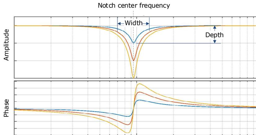
Parameters controlling the operation of notch filter are:
