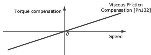
As the speed increase, so the viscous friction compensation increases with a rate defined by the Viscous Friction Compensation parameter.
