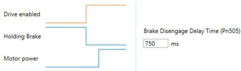
If Pn505 is a negative value, when the Servo ON command is received, the power will be supplied to the motor immediately, then the brake signal will change after the delay time.
