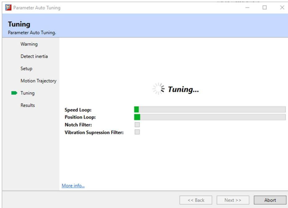
Results: Once the tuning process has completed, the calculated gain terms will be displayed with an option to save them to the drive.
