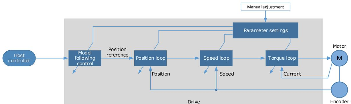
The Model Following Control function is enabled via Pn150.
