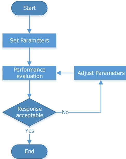
There are various indicators used to evaluate servo performance including bandwidth, response time, overshoot, steady state error, anti-load disturbance, speed ripple fluctuation, torque ripple, etc. The importance of these will depend on the application.
