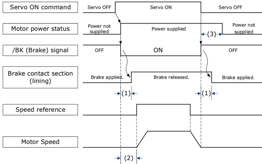
(1): The brake delay times for motors with Holding Brakes.
