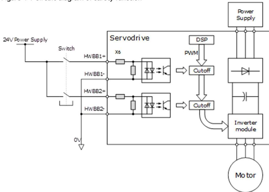
Close the Switch for turning ON HWBB1 and HWBB2, PWM signal can be allowed to pass by Cutoff circuit, which is, allowing the torque to output.
