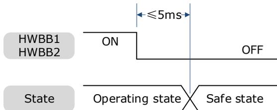
Safety output signal from the safety controller and safety sensor may include L pulse for self-diagnosis. Make sure the off period of safety input signal less than 1 millisecond, and the safety input circuit does not detect this OFF event.
