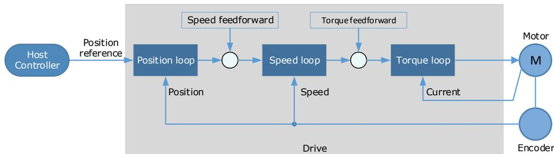
In general, the differential of the position reference is used as the feedforward. This is known as an internal feedforward reference and is the default mode of operation. Other options are available for generating the feedforward reference.
