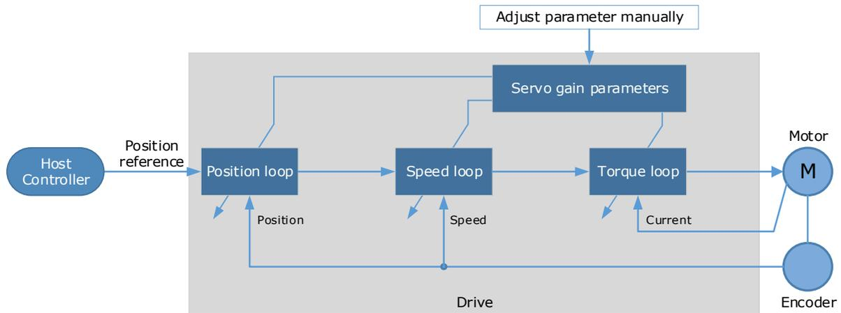
It is necessary to adjust the three-loop control parameters of the Servo from the inside out, that is, the adjustment sequence is **Torque loop** → **Speed loop** → **Position loop**. In order to maintain stability, the bandwidth setting should be the largest in the torque loop, then the speed loop, and the position loop should be smallest.
