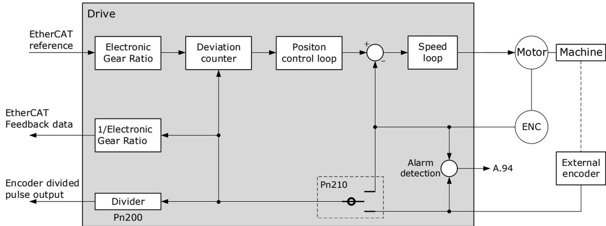
This setup can be useful in some high-precision positioning applications where there is compliance or backlash between the motor and the load.
