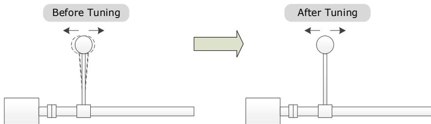
The aim of the Model Following Control is to maintain the stability of the load position based on a relationship between load position and Motor position. This is done by correcting the position reference and generating new speed and torque feedforward values.
