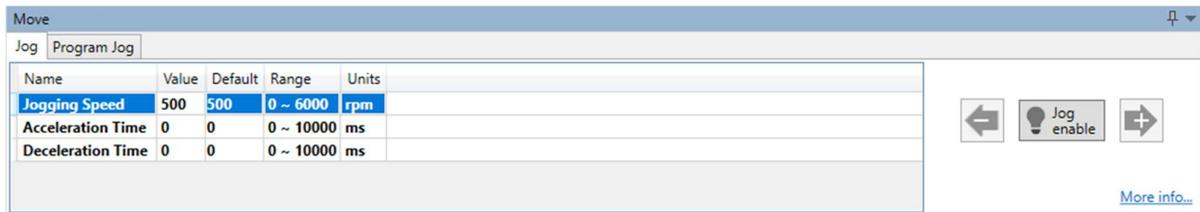
The motion profile is controlled three parameters:
