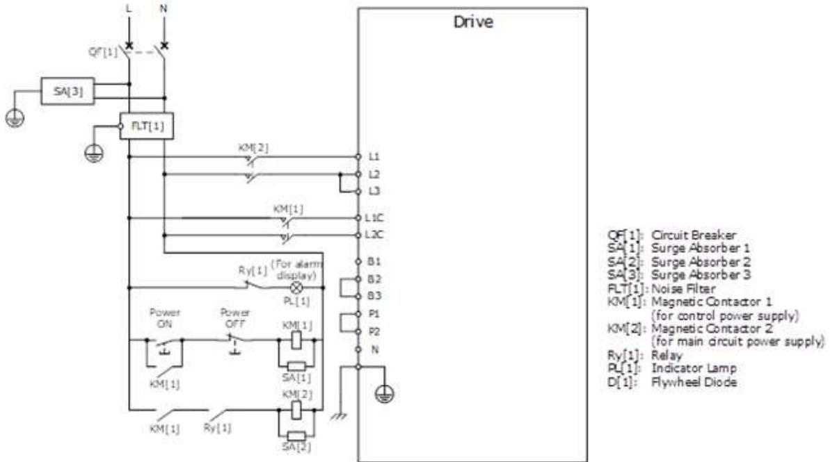
**NOTE:** for single phase wiring L or N can be wired into either L1 or L2
