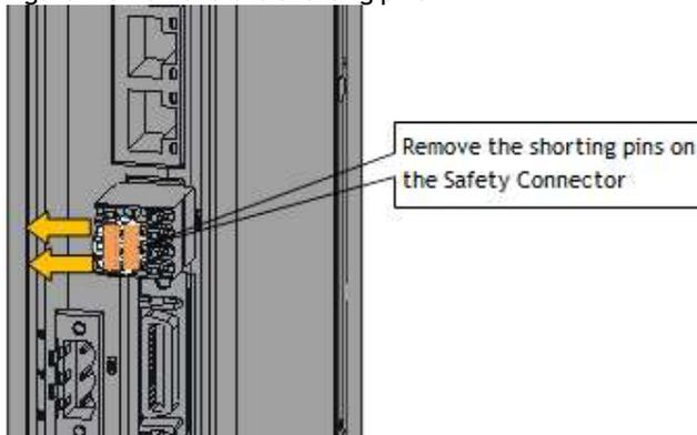
Step 2 Wiring the Safety Function Device
