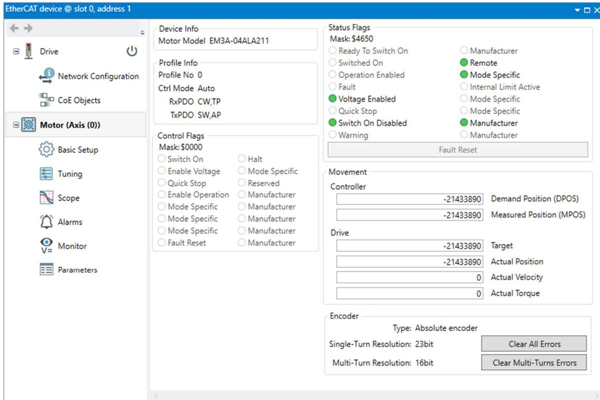
From any of the device configuration screens, for help or more information, pressing F1 will launch the Motion Perfect help based on the screen in view.
