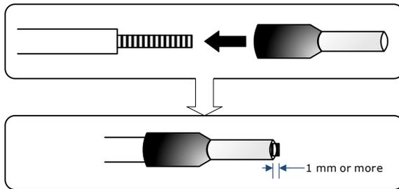
Step 4 Crimp the cable that has been inserted into the ferrule and cut off the cable conductor portion protruding from the ferrule (The allowable protruding length after cutting should not be more than 0.5 mm).
