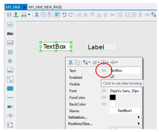
The menu then lets you choose what type of controller data to link to. This can be a program variable, for example in the program "MAINPROG" below, or VR, or other controller data types.
