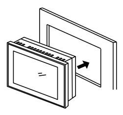
Insert the metal fixings supplied with the unit top and bottom. There are four mounting positions on the back of the Uniplay HMI unit, insert the fixing screws (included) and tighten them with a crosshead screwdriver.
