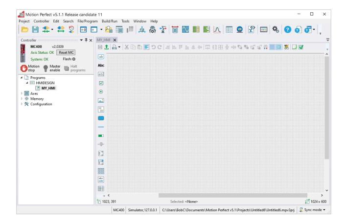
The components on the left-hand column can be dragged and dropped on the page.
