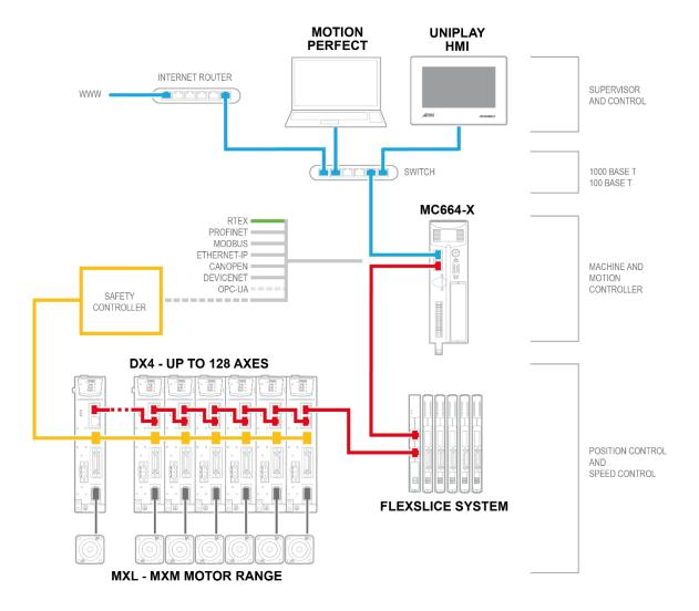
Once the application program is complete, the Uniplay HMI can be connected directly to the Ethernet port of the Trio Motion Coordinator.
