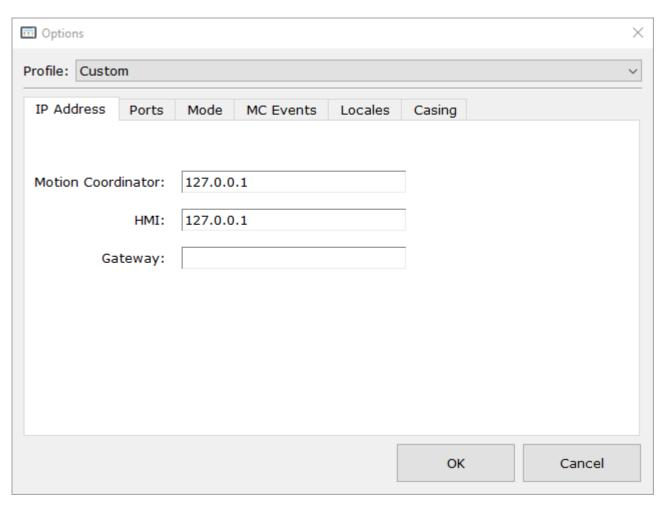
Once the IP address has been configured correctly, the Motion Coordinator will serve the pages to the simulator in the same was as it would to a real Uniplay HMI.
