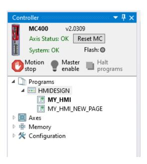
Note how one HMI screen is set to be the "Start-up page". This is the first page that will be displayed and is highlighted in bold in the program tree.
