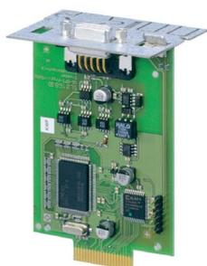
Accessory module for connecting PROFIBUS DP-V1.
