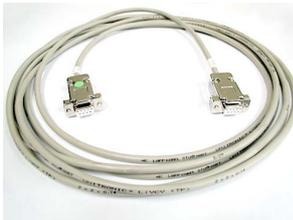
Description: Connection of inverter at terminal X3 and the PC, Sub-D connector, 9-pin, socket/ socket, approx. 5 m.
