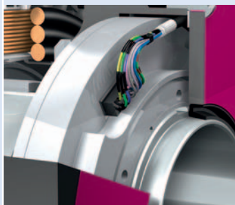
A single-turn absolute encoder with EnDat® protocol is used as the feedback system. Other encoders are available as an option.
