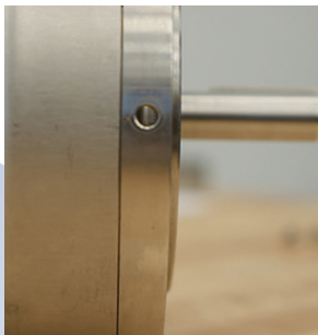
Weep holes on typical NEMA Motor
