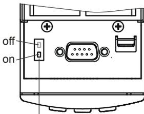
Internal terminating resistance 120 Ω can be activated
