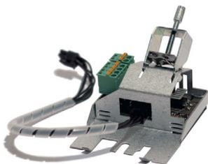
Accessory part for direct control of up to two motor holding brakes (24 V/DC). Attachable on the basic housing. Including connection cable for basic device and shield connection terminal for power cable cross-sections of 1 to 10 mm<sup>2</sup>.
