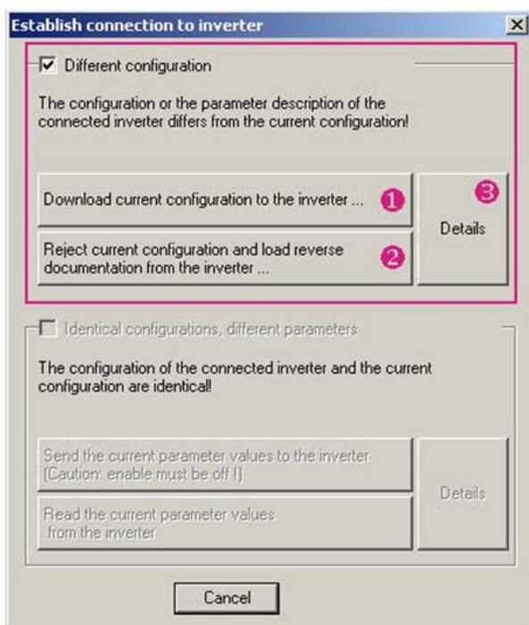
Fig. 7-3 Establishing connection with different configurations
