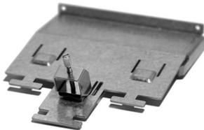
EMC shroud for size 3. Accessory part for shield connection of the motor line. Attachable on the basic housing. Including shield connection terminal for power cable cross-sections of 6 to 25 mm<sup>2</sup>. If necessary you can also connect the cable shield of the braking resistor and DC link connection on the shroud. Additional shield connection terminals are available as accessories for this purpose.
