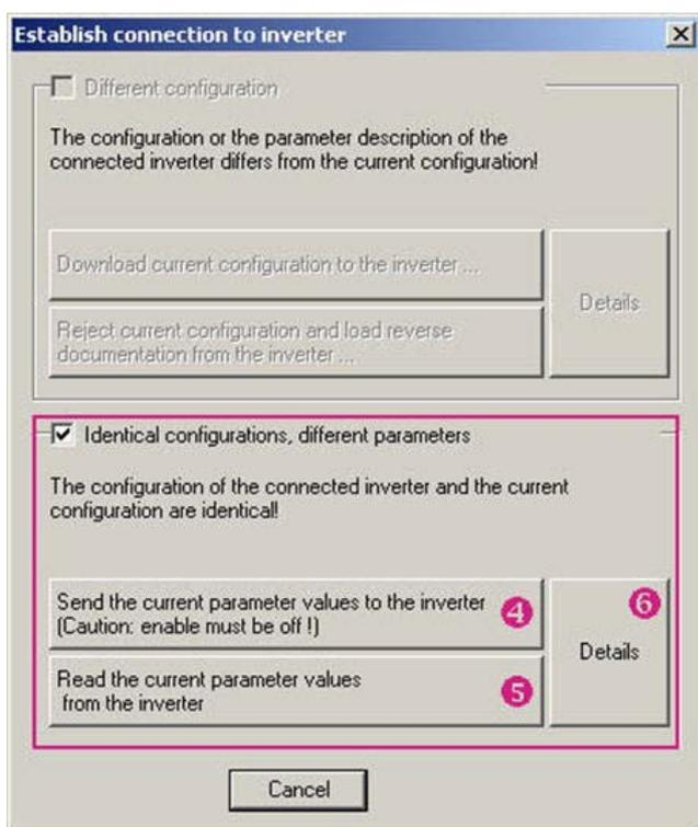
Fig. 7-4 Establishing a connection for identical configurations
