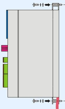
⇒ You have installed the submounting brake resistor.
