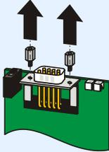
4. From below, thread the sub D plug connector of the PCB through the metal plate:
