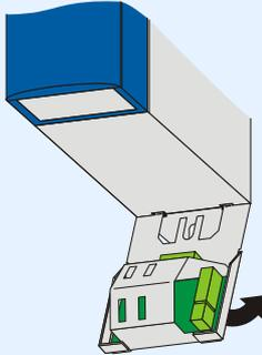
4. Attach the component to the mounting plate and inverter with the mounting screw and the washers:
