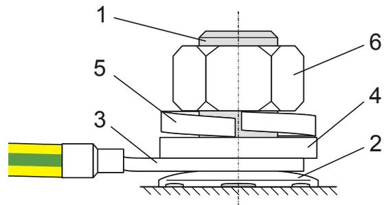
Contact disk, washer, return spring and nuts are supplied with the inverter.
