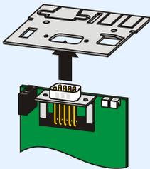
5. Secure the PCB to the metal plate with the screws which you removed in step 3:
