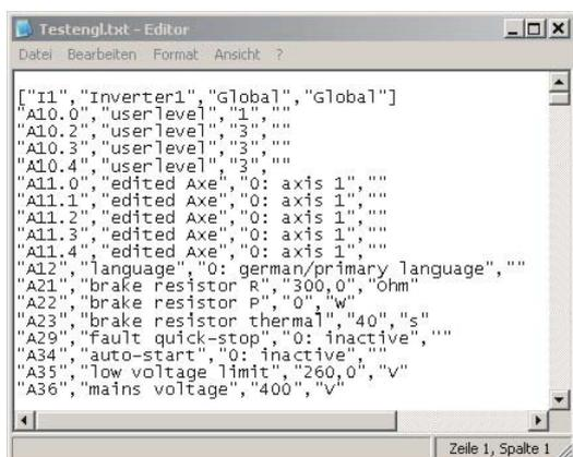
Fig. 9-2 View of exported parameters in CSV format
