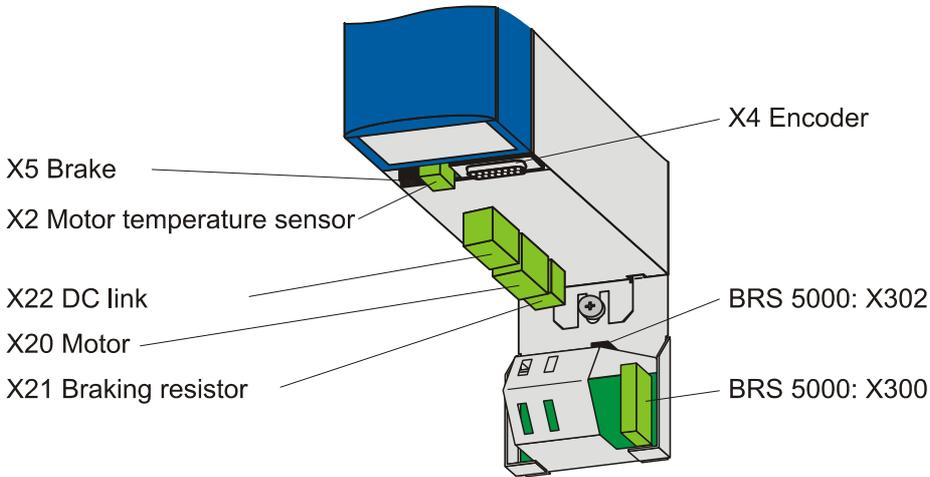
**Bottom of the device with BRS 5001**
