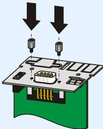
6. Guide the option board into the inverter so that the gold contacts slide into the black connector:
