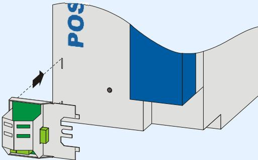
3. Secure the component to the device with the mounting screw and the washers:
