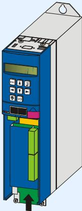
6. Secure the accessory part to the inverter with the mounting screws:
