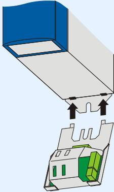
3. Press the back of the component onto the wall of the switching cabinet:
