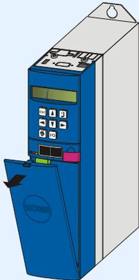
3. Lift the cover up and remove it from the inverter:
