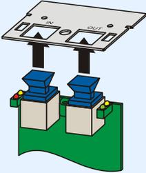
3. Secure the metal plate on the PCB with the included screw with locking disk:
