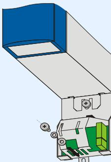
The attachment of brake module BRM 5000 or BRS 5001 to inverters of size 3 is different to the attachment to inverters of size 0 to 2.
