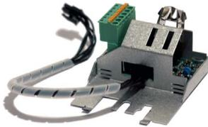
Accessory part for direct control of up to two motor holding brakes (24 V/DC). Attachable on the basic housing. Including connection cable for basic device and shield connection terminal.
