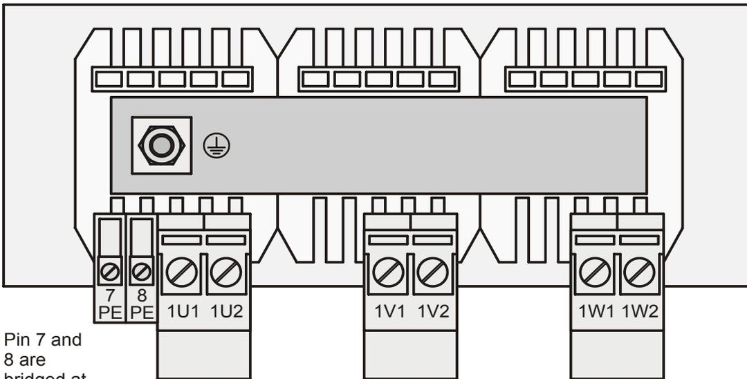
Pin 7 and 8 are bridged at the output derator
