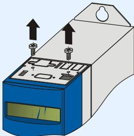
2. Remove the metal plate punch-out with a pair of pliers:
