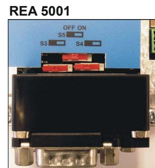
Please note that the switches are installed in different positions on the REA 5001 and XEA 5001 accessories. Identification of the switches and assignment of the switch positions to the function (switched on/switched off terminal resistance) are shown on the PCB cover.
