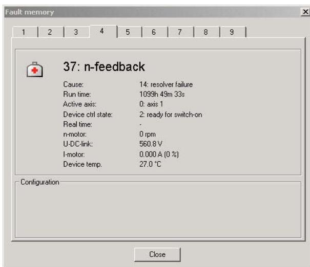
Fig. 8-1 View of the fault memory
