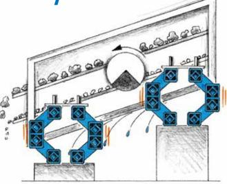
Vibration absorbing mounts for circular and linear motion screens
