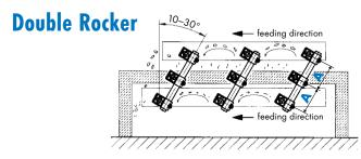
The three AR mountings are inserted on the round connecting tube (please check required material thickness by the relevant center distance on below-mentioned table). The counter-mass can be used as second trough with identical feeding direction.
