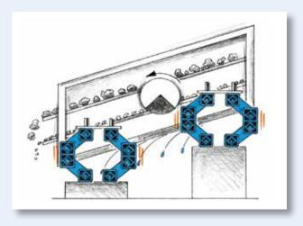
Circular motion screens or circular vibrators are normally excited by unbalanced weights that create a circular rotating oscillation of the screening frame. Relatively low accelerations of the screened material are achieved with this form of excitement. Circular vibrators thereby normally work with a screening frame inclination of 15° to 30°, so that an adequate material throughput is ensured.
