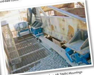
Circular motion screen for gravel on AB TWIN Mountings
