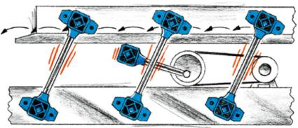
Rocker arms and drive heads for crank shaft driven shaker conveyors
