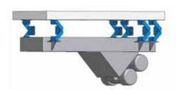
Discharge chutes under silos are normally supported by means of complicated yoke constructions and are suspended on pressure springs. With its HS suspensions (HS = hanging screen), ROSTA offers the possibility of the direct, costeffective suspension of the discharge unit on silos and bunkers. The geometry of the HS suspensions has been designed to accommodate tensile loads.
