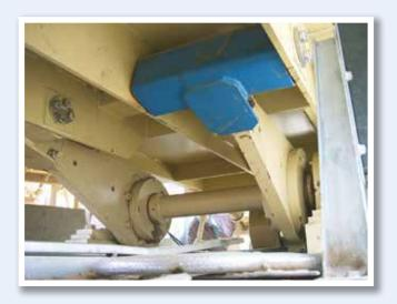
The biggest standardized ROSTA drive head type **ST 80** is laid out to transmit acceleration forces up to 27'000 N on shaker troughs. For the actuation of e.g. heavy feeding hoppers or very long wood-waste shaker conveyors this capacity is not sufficient.
