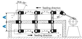
The three AR mounts are inserted on the round connecting tube, with the direction inverted center element. This so said "boomerang"-configuration is offering on the counter-mass trough a direction inverted flow of material, what could simplify selection and screening processing.
