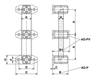
Type AD-PV with inverted flange
