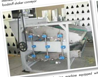
Two-directional acting seed cleaning machine equipped with AR-"Boomerang" double rocker arms
