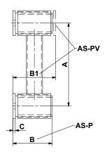
Type AS-PV with inverted flange
