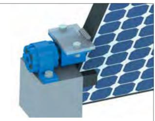
Example of an element connection in series ( $\pm60^{\circ}$  element torsion) as strong wind swivel mount for solar panels, consisting of a series connection DW-C and DK-C elements with BK bracket.
