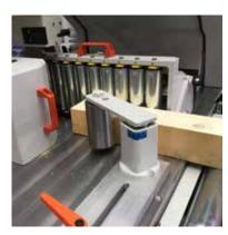
Tensioner devices with a  $\ensuremath{\text{pressure roller}}$
