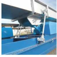
Conveying and screening trough for **wood** splinters
