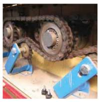
Tensioner devices for chain drives on **loading stations**
