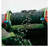
Suspension for belt scrapers on conveyor belts
