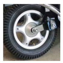
Rubber suspension for the **wheel** suspension
