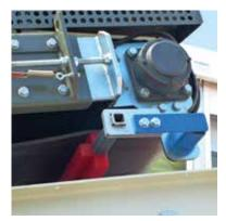
Tensioner device for conveyor belt scrapers
