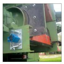
Rubber suspension element for **conveyor belt scrapers**
