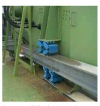
**Counter-oscillating frame mounting** for a vibrating screen
