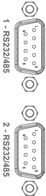
COM Port 1 is assigned to communications channel #1 in Motion Perfect and COM Port 2 is assigned to channel #2 by default. Additional information about using the serial ports can be found in the help file for the “print” command.
