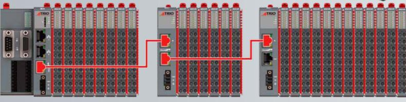
Up to **16 MS I/O slices** can be connected via **MS-Bus** to a single **MS EC Coupler** in any combination. Multiple couplers can be connected to a single EtherCAT controller for complete machine control.
