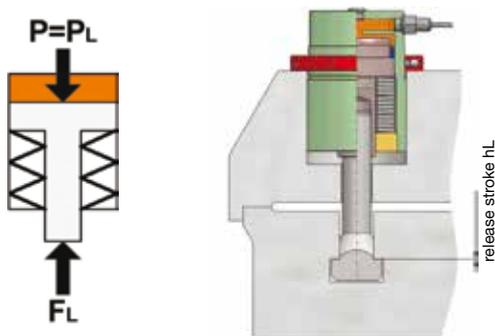
load with release pressure  $P_L$ , disk spring package is compressed further
