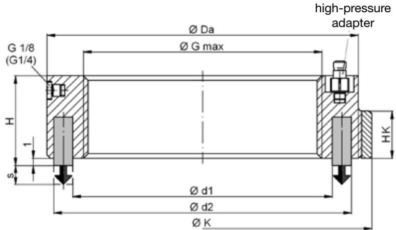
Technical data and dimensions [mm]: length dimensions according to DIN ISO 2768 mH
