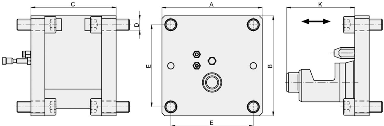
Technical data and dimensions [mm]: measure of length according to DIN ISO 2768 mH
