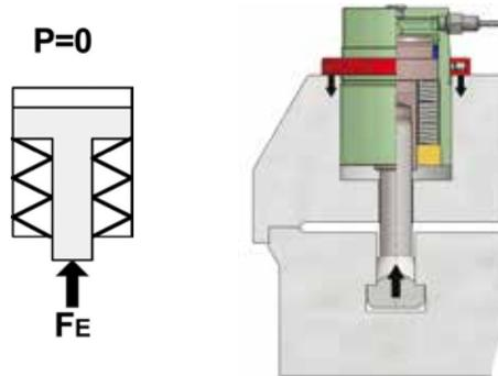
release hydraulic pressure -  $P = 0$  bar - clamping force of disk spring package =  $F_N$
