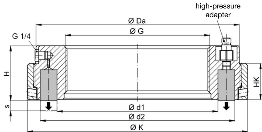
Technical data and dimensions [mm]: length dimensions according to DIN ISO 2768 mH
