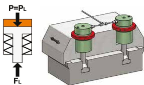
T-bolt screw and tensioning bolt are in release position. Slide can be moved axially
