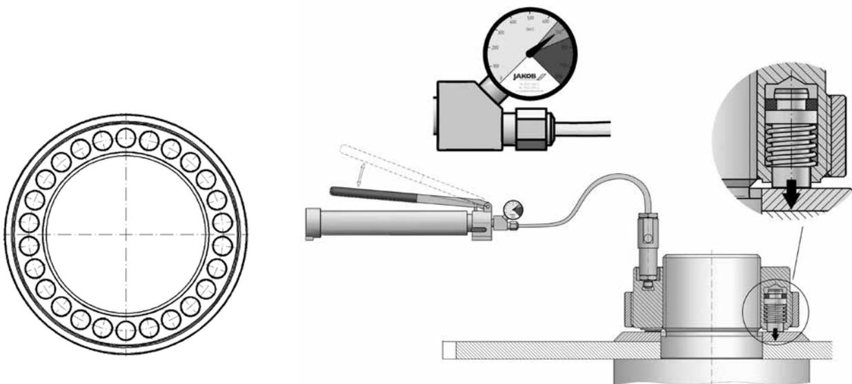
The JAKOB multi-piston system is a genuine innovation in the hydraulic clamping sector. The main design feature is a ring-shaped cylinder housing with internal threads. Several small thrust pistons are arranged concentrically on its base. The individual piston bores are connected hydraulically using a special tangential recess. A patent has been registered for this principle.
