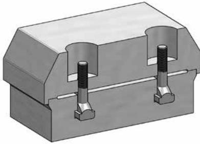
T-bolt screw or tension bolt installation (consider twist lock)
