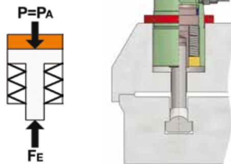
load cylinder with adjusting pressure  $P_A$  - disk spring package is compressed - T-bolt screw is released by stroke of pressure piston
