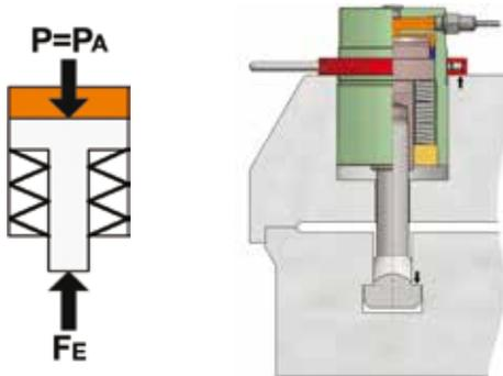
turn ring nut until ring nut and tensioning bolt are at mechanical stop - lock ring nut with screw
