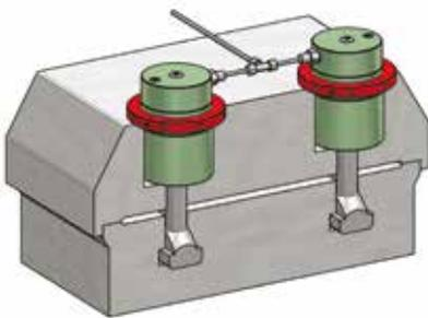
installation of cylinder, hydraulics -> bleeding of cylinder
