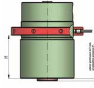
adjust ring nut to mounting position (M) and lock
