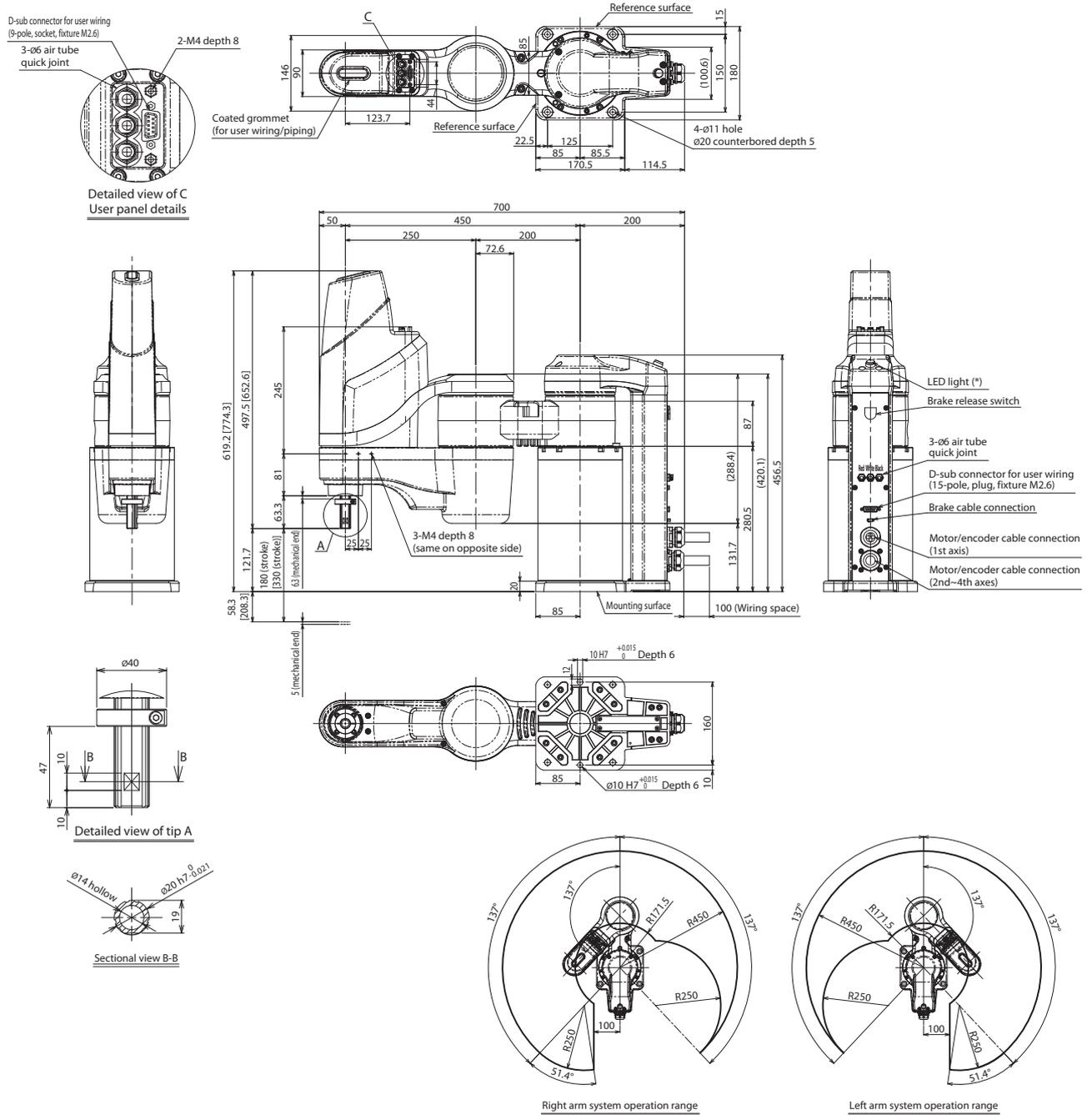
(\*) To operate the LED, wire a controller output to apply 24VDC to the LED terminal of the user wiring.
