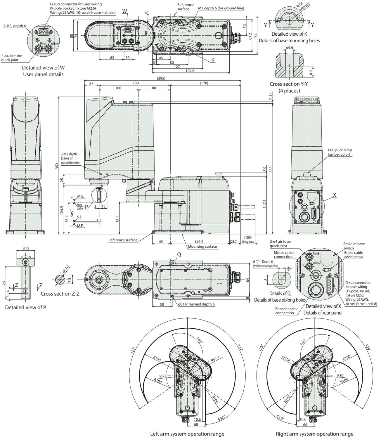
(\*) To operate the LED, wire a controller output to apply 24VDC to the LED terminal of the user wiring.
