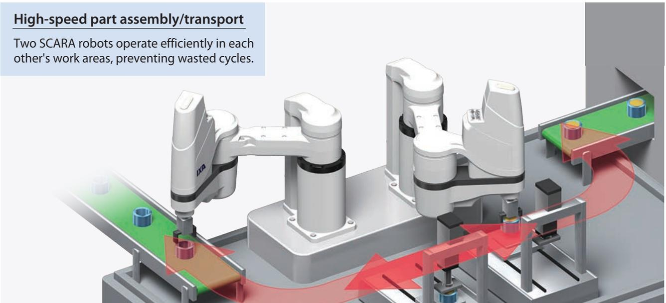
**High-speed pick and place of radiators and chips**
