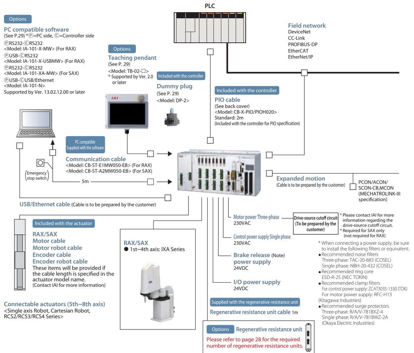
(Note) When connecting an actuator with brake, the brake power supply +24V is required for the controller.
