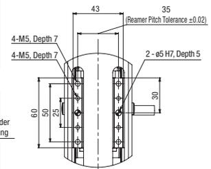
Detailed Diagram U (Detail of Z-axis Slider)
