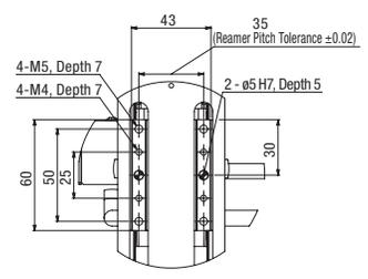
Detailed Diagram V (Detail of Z-axis Slider)
