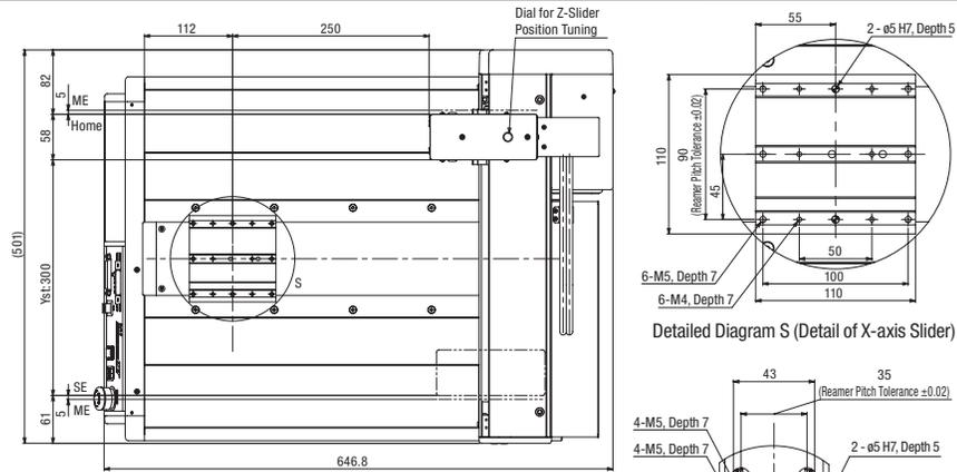
Detailed Diagram S (Detail of X-axis Slider)
