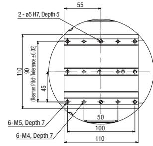
Detailed Diagram S (Detail of X-axis Slider)
