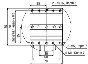
Detailed Diagram U (Detail of Y-axis Slider)
