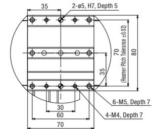
Detailed Diagram U (Detail of Y-axis Slider)
