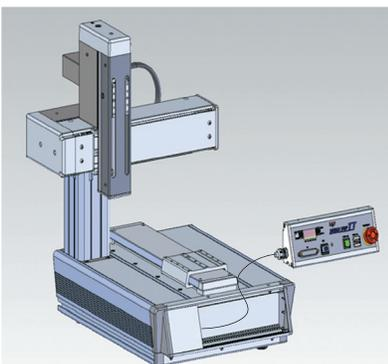
The operation console can be separated from the product for handy operation.
