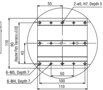
Detailed Diagram S (Detail of X-axis Slider)
