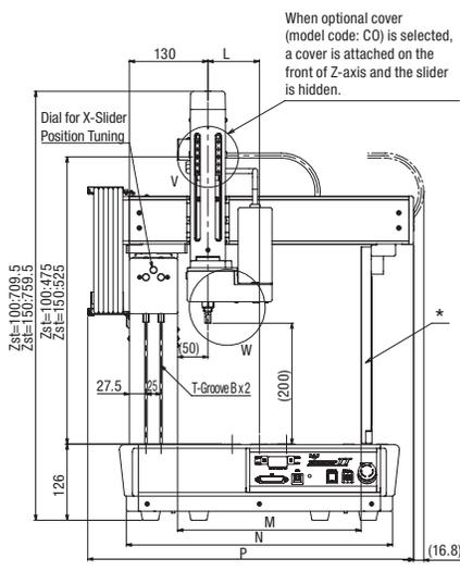
When optional cover (model code: CO) is selected, a cover is attached on the front of Z-axis and the slider is hidden.
