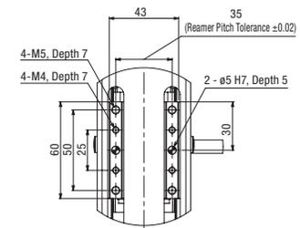
Detailed Diagram U (Detail of Z-axis Slider)
