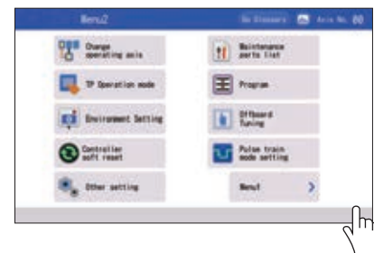
Pressing and holding the bottom right section of the screen allows you to take screen shots.
