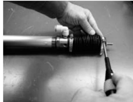
Tightening of front metal fitting
