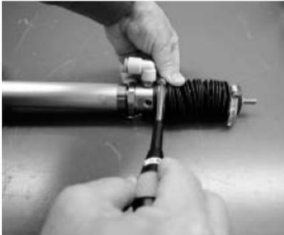
Tightening of rear metal fitting
