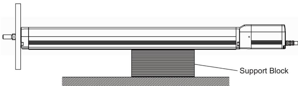
Operation of the actuator with attachment only on the front bracket and the front flange (option) applies the external force of the acceleration / deceleration multiplied by the weight of the actuator to the unit body.
