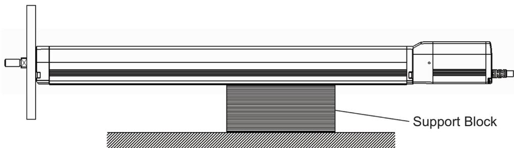
Operation of the actuator with attachment only on the front bracket applies the external force of the acceleration / deceleration multiplied by the weight of the actuator to the unit body. Control the acceleration / deceleration at 0.05 G or less (for reference) when the actuator of RA8 or RA10 is moved with attachment only on the front bracket.
