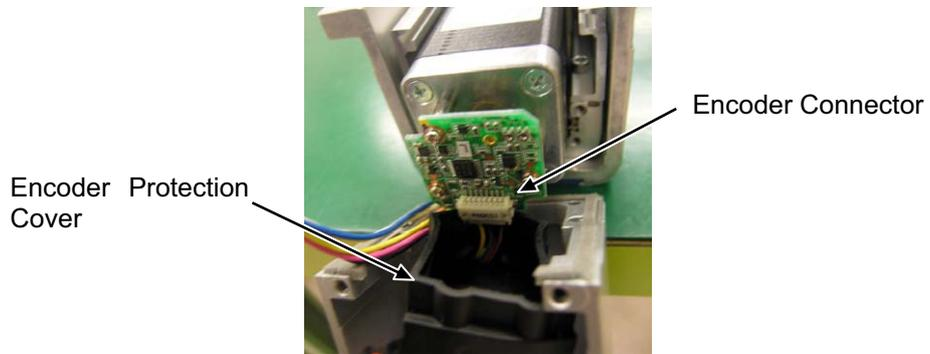
19) Put the encoder protection cover on the encoder.
