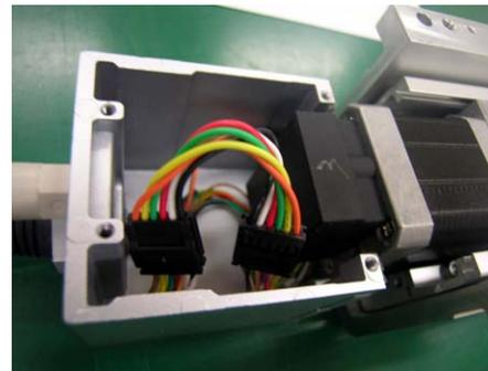
21) Insert a hex wrench to the holes the grommets were taken out of to tighten the four hex socket head cap screws to hold the motor cover (at the circled places) with it.
