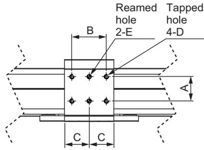
Reamed Hole Pitch Tolerance:  $A \pm 0.02$
