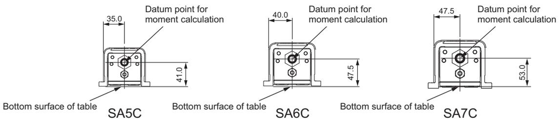
**⚠ Caution:** An operation beyond the allowable moment and overhang load length would not only generate abnormal noise and vibration, but also may shorten the life of actuator extremely.
