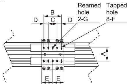
Reamed Hole Pitch Tolerance:  $A \pm 0.02$
