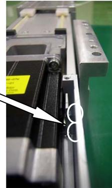
13) By using a tool with a long and slim shape such as a hex wrench, push in the four grommets (at the circled places) on the back.
