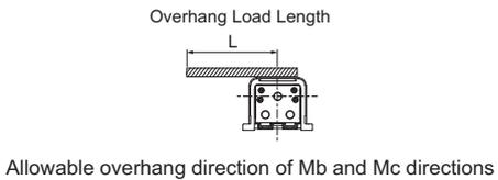
If installing on the top surface of the slider, for the calculation of  $M_a$  and  $M_c$  moments, consider the position indicated with an arrow as the datum point.
