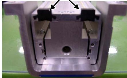
3) Tighten the four hex socket head cap screws to hold the cover on the side opposite to the motor (at the circled places) with a hex wrench to attach the cover.
