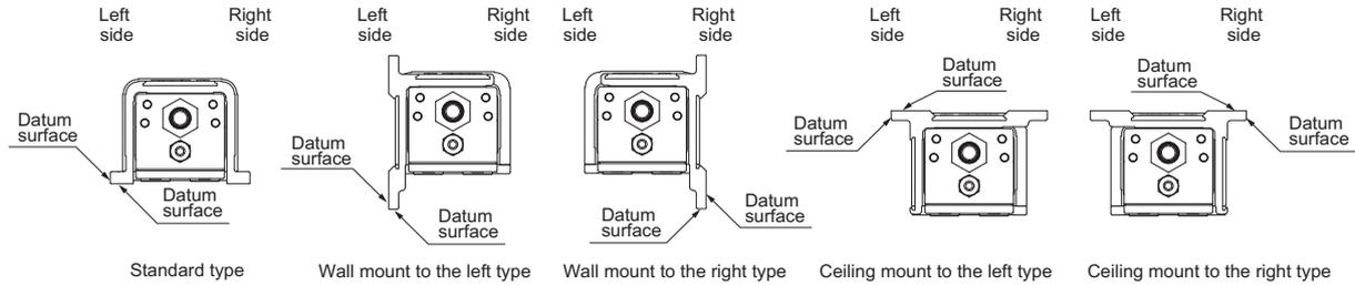
Positions of Datum Surfaces (View from Shaft End on Motor Side)
