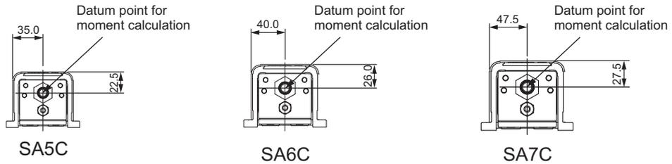
If installing on the bottom surface of the slider, for the calculation of  $M_a$  and  $M_c$  moments, consider the position indicated with an arrow as the datum point.
