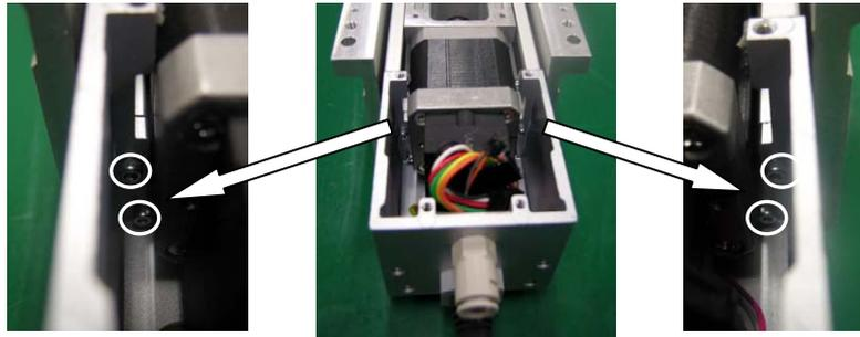
22) By using a tool with a long and slim shape such as a hex wrench, push in the four grommets (at the circled places) on the back.
