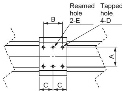
Reamed Hole Pitch Tolerance:  $A \pm 0.02$
