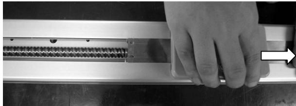
(6) After the stainless steel sheet passes through the slider, pull one end of the stainless steel sheet out to the position of the stainless steel retainer plate.
