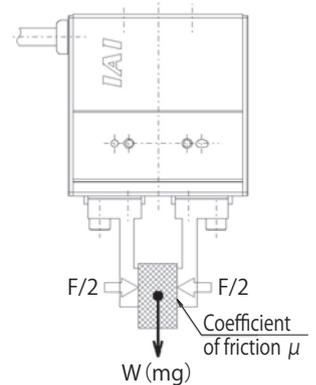
\* The greater the coefficient of static friction, the greater the maximum allowable work part mass becomes. To ensure safety, however, select a model that can generate a gripping force of at least 10 to 20 times this work part mass.
