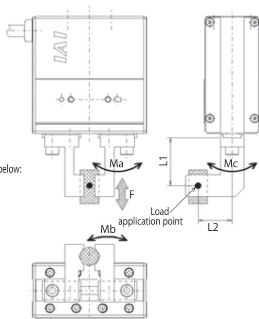
\* The load application point shown above indicates the position of the load applied to the finger. This position varies depending on the type of load.
