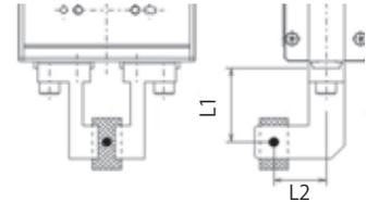
\* Operate with the L1 distance under 20 mm.
