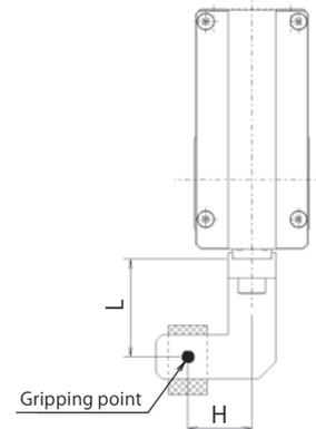
Even when the gripping point distance is within the limits, still design your actuator as compact and lightweight as possible. If the finger is long and large, or heavy, the inertial forces generating upon opening/closing as well as bending moments may cause the performance of the actuator to drop or negatively affect its guide.
