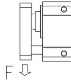
\* Single-guide specifications can only be used with vertical loads.
