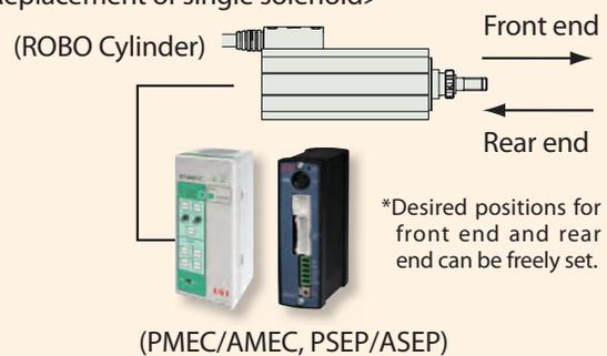
\*Desired positions for front end and rear end can be freely set.
