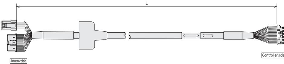
Minimum bend radius  $r = 68\text{mm}$  or larger (when movable unit is used)
