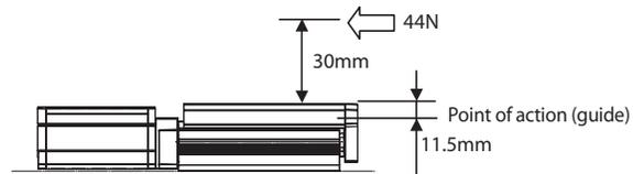
The TA4C allowable dynamic moment ( $M_a$ ) is 4.2 (N·m), which means 80% is 3.36.
