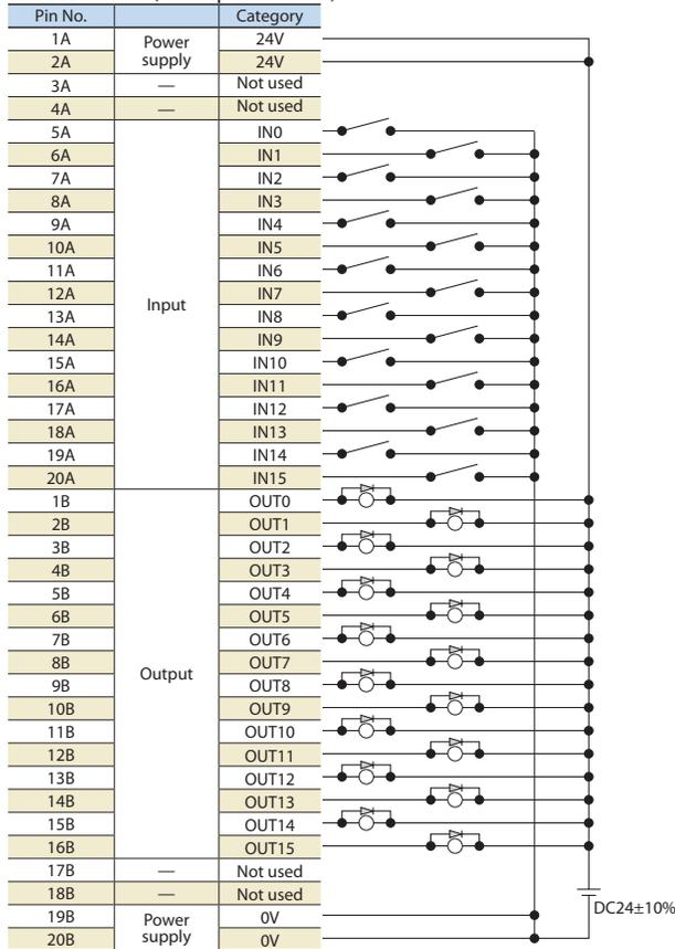
\*Connect Pins 1A and 2A to 24V, and Pins 19B and 20B to 0V.
