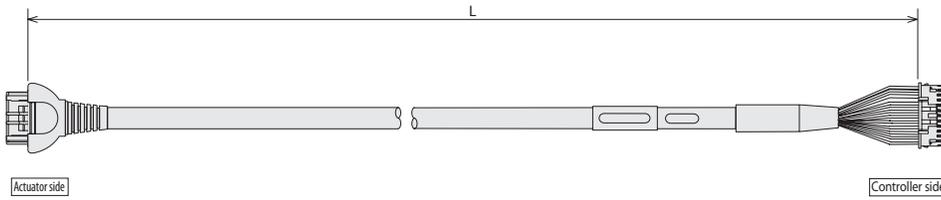
Minimum bend radius  $r = 68\text{mm}$  or larger (when movable unit is used)
