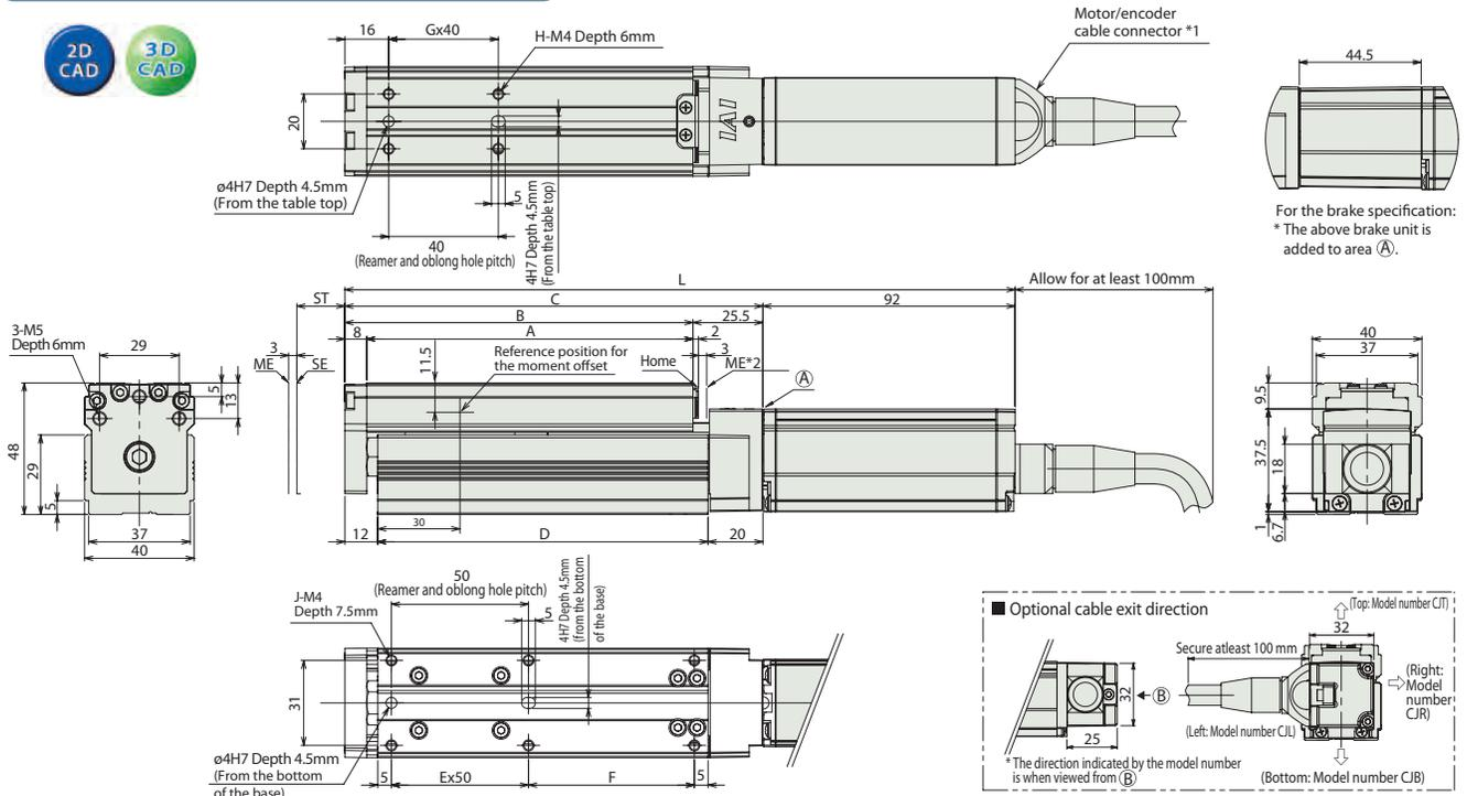
\* 1 The motor-encoder cable is connected directly to the actuator motor cover.
