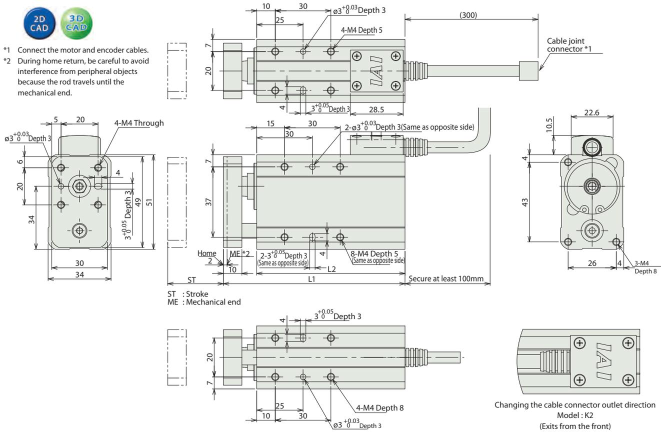
Changing the cable connector outlet direction
