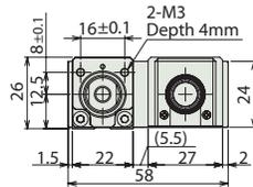
Dimensions of nut at tip of rod
