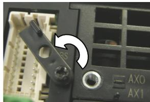
[Step 3] Grab the lattice\* on the fan unit with a tool such as needle-nose plier, and pull out the fan unit.
