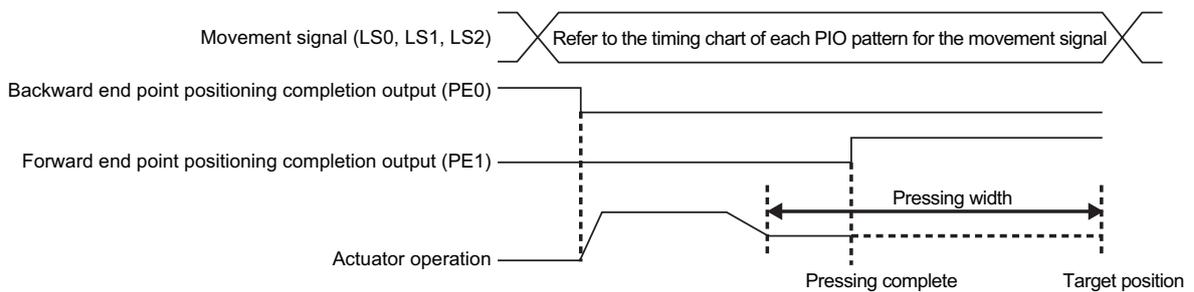
**Caution:** For the pressing operation, use the positioning complete signal (PE\*). Even the operation finishes with a miss-pressing and reaches the end point, PE\* signal will turn ON. Set the pressing width wider when miss-pressing detection is required and identify with a timer.
