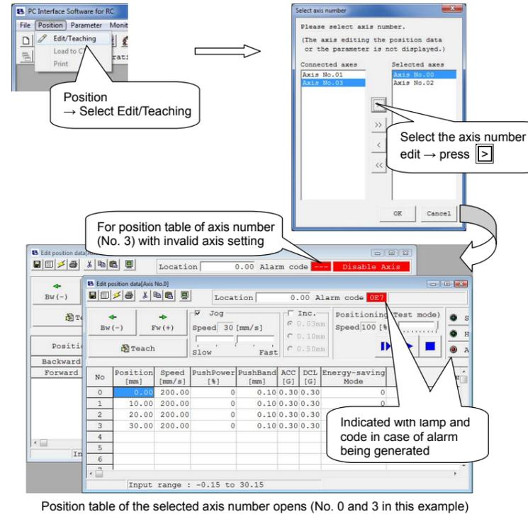
**Caution:** If there are only two to three areas of the lines to input the position for the open position table, conduct Steps 1 to 4 in 3.2.2 "Initial Setting" of MSEP Instruction Manual to establish the settings in Operation Pattern 6.
