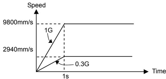
**⚠ Caution:** (1) Set the speed, acceleration and deceleration so that they do not exceed the rating values described in the brochure or the instruction manual of the actuator. The setting that exceeds the rated acceleration/deceleration speed may shorten the actuator life remarkably.
