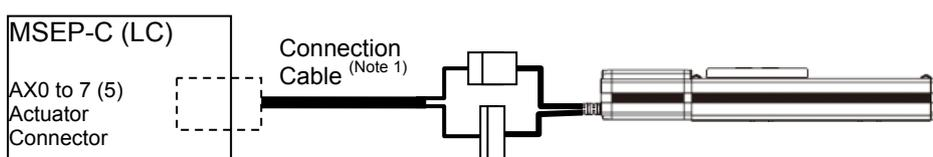
Note 1 Applicable Connection Cable Model Codes □□□: Cable length Example) 030 = 3m
