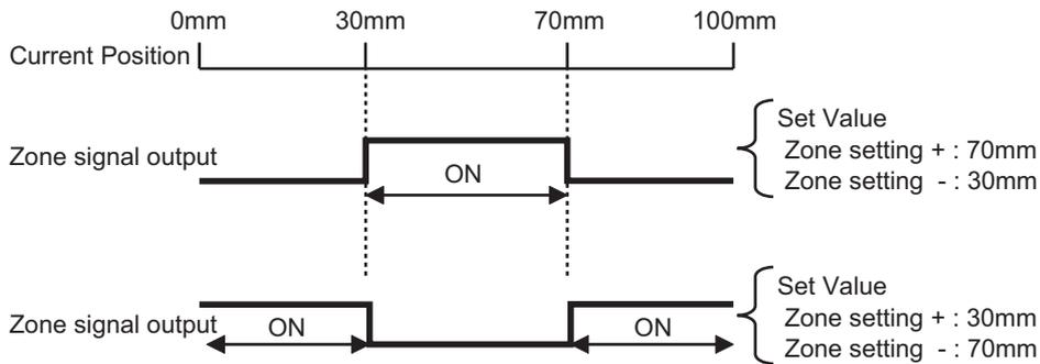
**⚠ Caution:** The signal cannot be output unless the range of the zone detection is set to a value greater than that of the minimum resolution (actuator lead length/encoder resolution).
