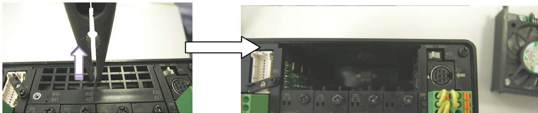
[Step 4] The new fan unit is to be pushed in to be settled. At this time, make sure the fan unit is pushed in down to become flush with the peripheral.
