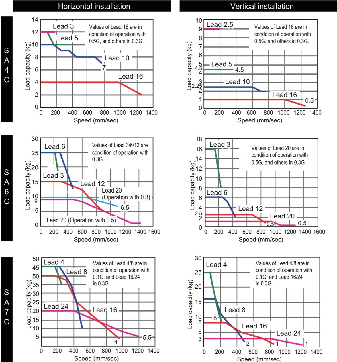
Correlation diagram of speed and loading capacity for the RCP5 slider type
