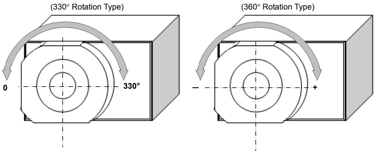
For 360° Rotation Type with the origin reversed type, the directions of + and - are the other way around.
