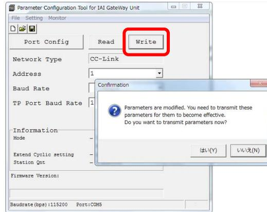
[Step 12] After rebooting, a confirmation window for parameter reading appears for confirmation of the written contents. Click “Yes” to accept the reading.
