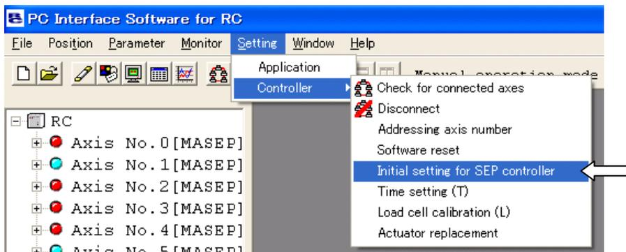
[Step 3] Select the axis number which the setting is to be conducted.
