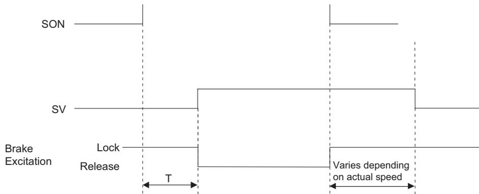
$$T \text{ (before detecting excitation)}^{(\text{Note})} = \text{SON signal identification (7ms)} + \text{Excitation detection time (Parameter No.36=0 : 170ms, No.36=1 or 2 : 220ms)} \times \text{Number of retry (10 times Max.)} + \text{Servo ON delay time (20 (Pulse motor), 50 (Servo motor) ms)}$$
