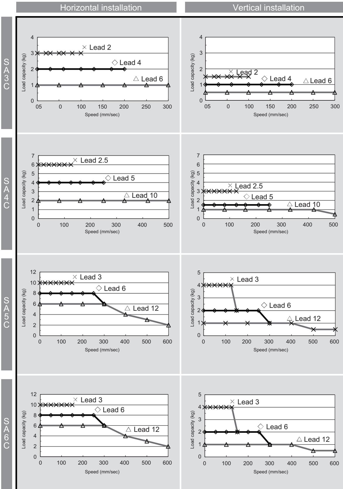
Correlation diagram of speed and loading capacity for the RCP3 table type
