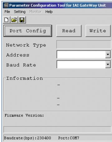
[Step 4] Reading is started from MSEP to PC. Click on the “Read” button and a confirmation window appears. Click on the “Yes” button. Once the parameter reading is completed in normal condition, the reading complete window opens. Click OK.
