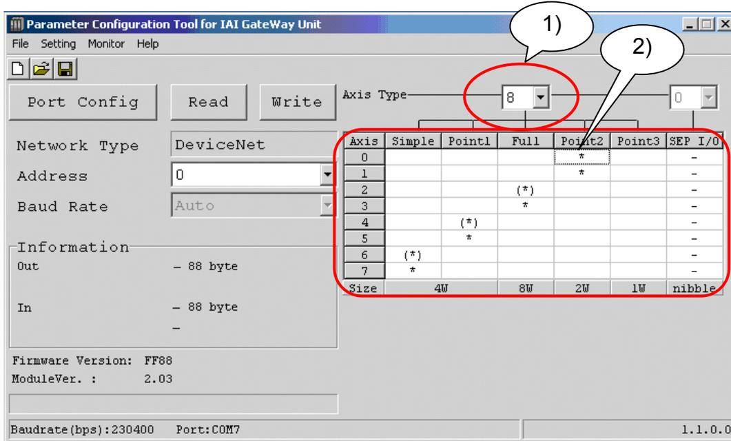
When selecting the operation mode, select the axis number in the pull down menu circled as 1). By selecting the number, the cells in 2) become blank in response. Click the cell for the mode to be set in each axis.
