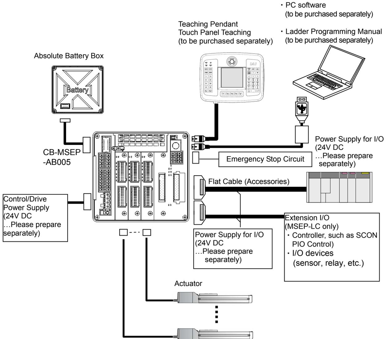
**Caution:** Make sure to turn the power to the controller OFF when inserting or removing the connector that connects the PC software or teaching pendant to the controller. Inserting or removing the connector while the power is turned ON causes a controller failure.
