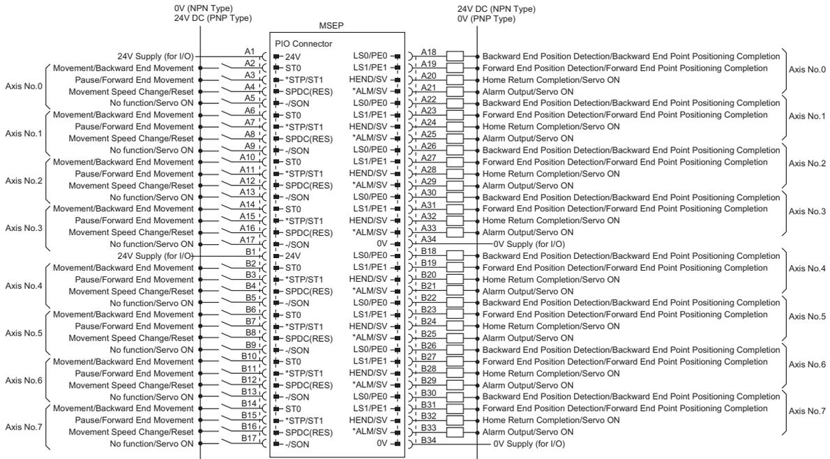
“\*” in codes above shows the signal of the active low. Processing occurs when an input signal of the type is turned OFF. An output signal of the type is normally ON in the power-on status and turned OFF at signal output.
