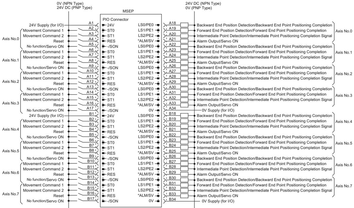
“\*” in codes above shows the signal of the active low. Processing occurs when an input signal of the type is turned OFF. An output signal of the type is normally ON in the power-on status and turned OFF at signal output.
