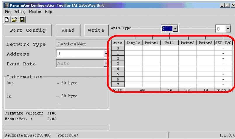
[Step 15] Click on a blank cell and "\*" shows up. "\*" mark means that an operation mode is selected for each axis.
