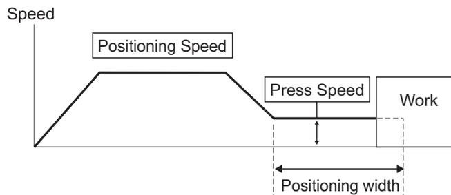
**⚠ Caution:** If the speed of the positioning of the position table is set below this parameter, the pressing speed will become the same as the positioning speed.
