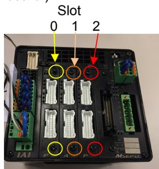
The figure shows the 6-axis type. (Slot 3 is located beside Slot 2 for 7 and 8-axis types.)
