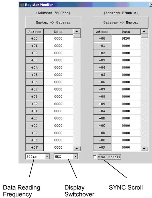
In this register monitor window, shows the data that Gateway Unit has received from the host (master) and the data sent back to the host (master).
