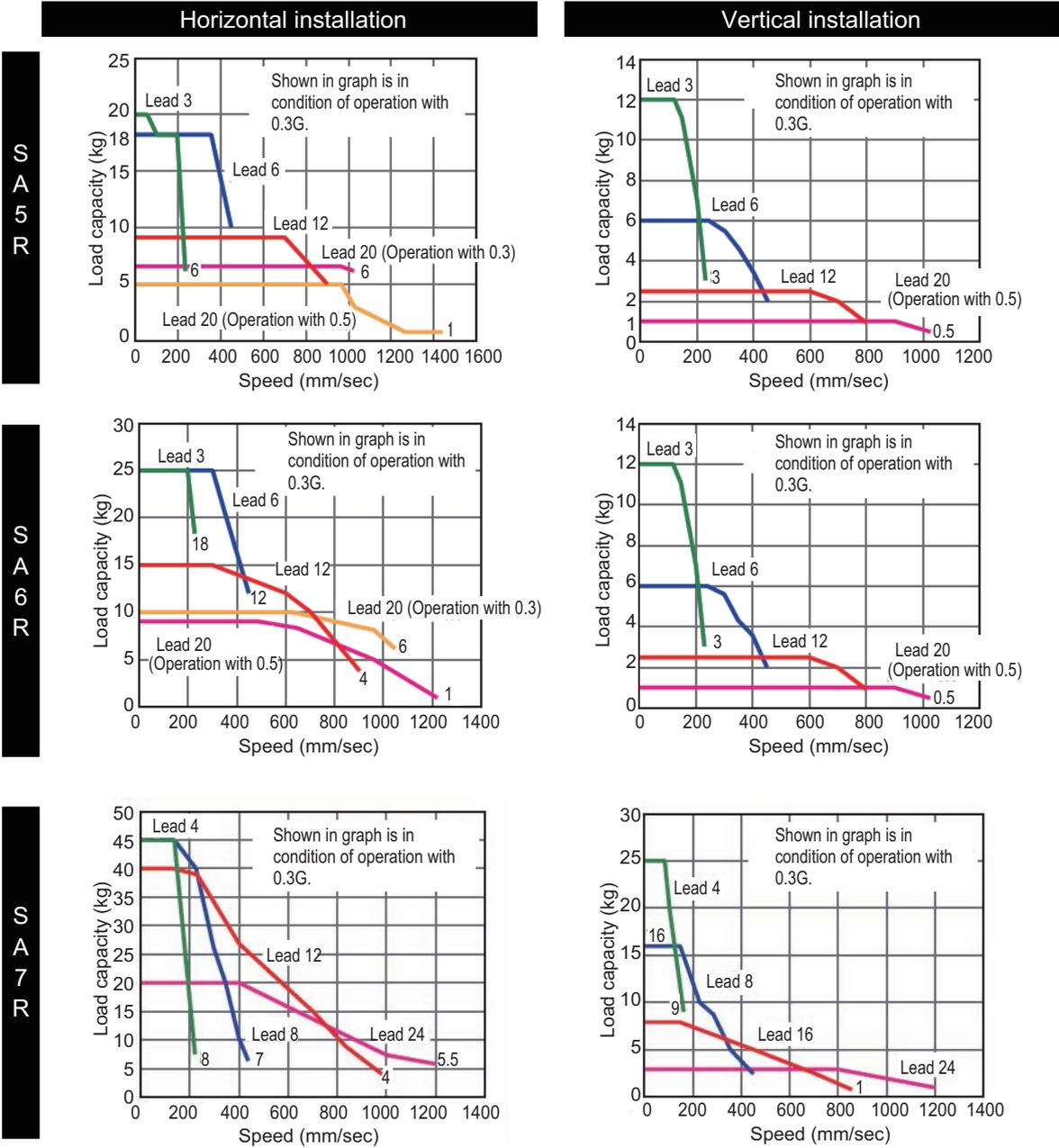
Correlation diagram of speed and loading capacity for the RCP4 rod type
