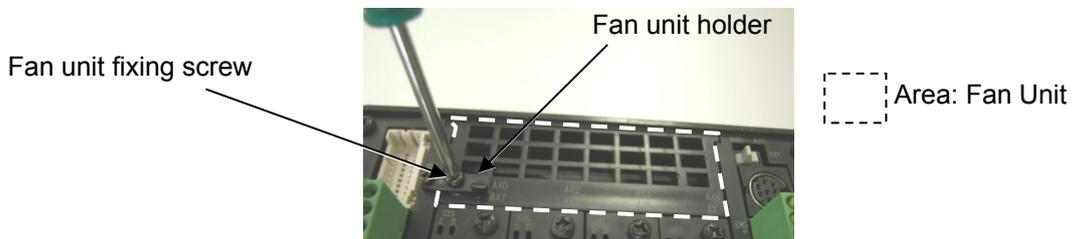
[Step 2] Rotate the fan unit holder till it goes out of the fan unit interference.
