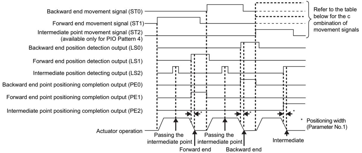
Following table shows the combination of the movement signals by each PIO pattern and the destination determined by it.
