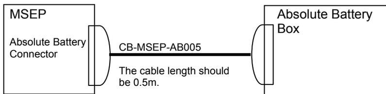
(Note) Do not apply force not being perpendicular to the connector when insert or detach the cable.
