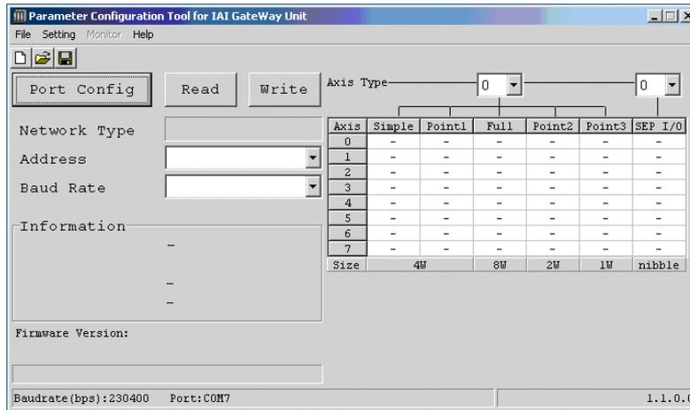
[Step 11] Reading is started from MSEP to PC. Click on the “Read” button and a confirmation window appears. Click on the “Yes” button. Once the parameter reading is completed in normal condition, the reading complete window opens. Click OK.
