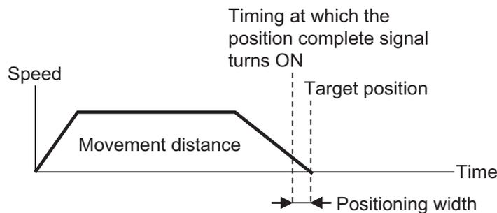
When the servo-motor is turned ON from OFF condition, the positioning is performed with the position set as the target position. Accordingly, this signal is turned "ON" and after that, when the positioning operation is started with the home return (HOME) signal and positioning start (CSTR) signal, this signal is turned "OFF".
