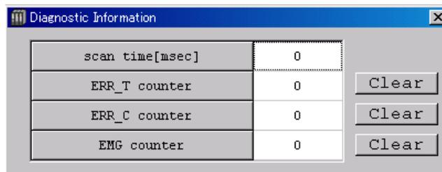
The number of the communication error (ERR\_C and ERR\_T) occurrence and number of the emergency stop (EMG) detection can be counted.
