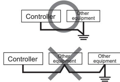
Do not share the ground wire with or connect to other equipment. Ground each controller.
