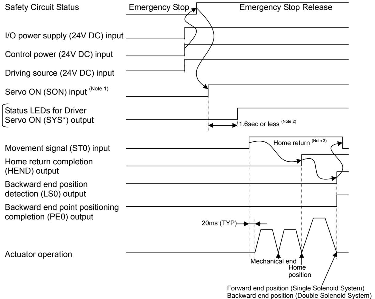
Note 1 When the servo control is set to "Use" in the initial setting, the servo is turned ON by means of inputting the SON signal.
