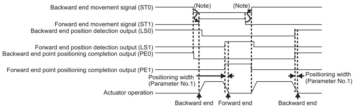
(Note) When having a movement command, make sure to turn OFF both ST0 and ST1 before issuing a movement command to the target position.
