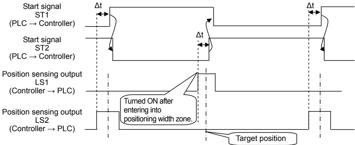
$\Delta t$ : Time required to certainly reach the target position after the position sensing output LS1 or 2 is turned ON.
