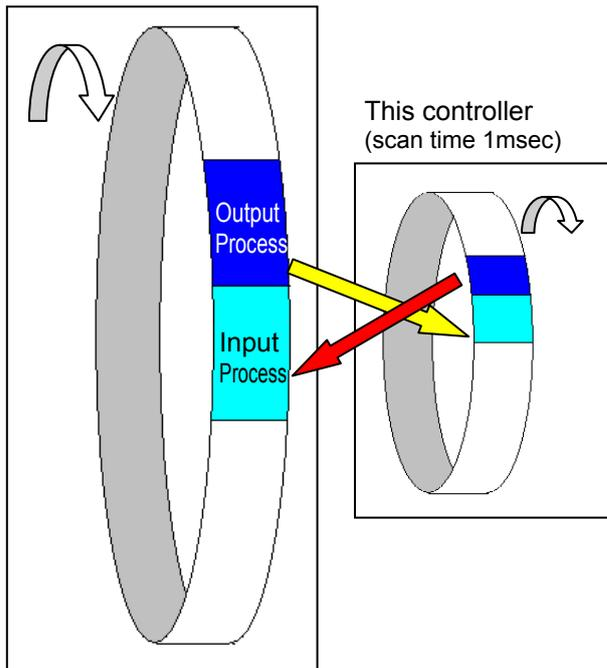
As shown in the diagram, the input and output timings of two devices that have different scan time do not match, when transferring a signal. There is no guarantee that PLC would read the signal as soon as this controller signal turns ON. In such a case, make the setting to read the signal after a certain time that is longer than the longer scan time to ensure the reading process succeeds on the PLC side.
