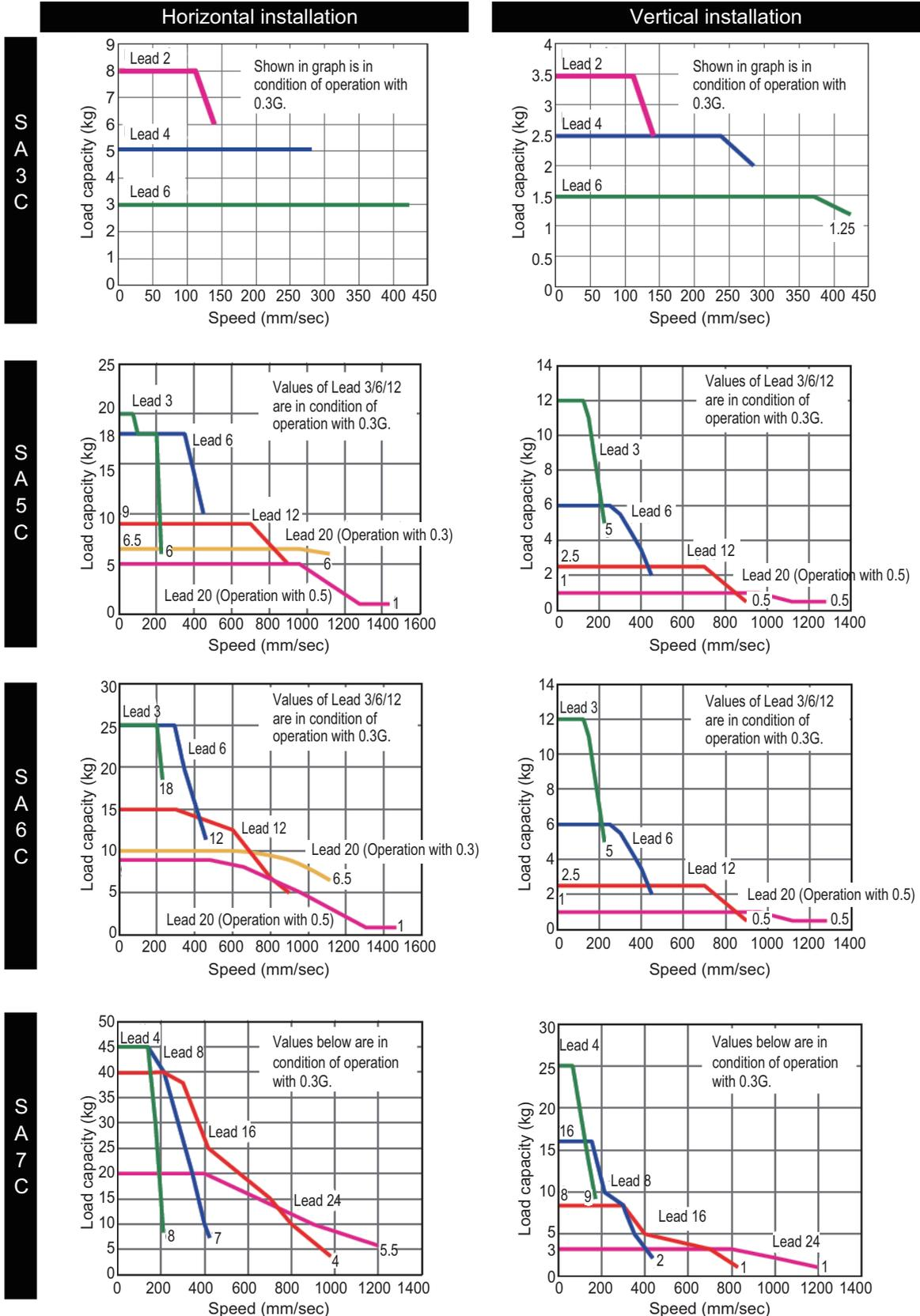
Correlation diagram of speed and loading capacity for the RCP4 slider type
