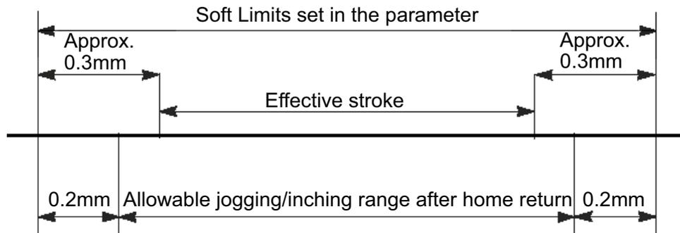
The operational range of JOG or Inching after a home-return operation is 0.1mm (deg) outside the set area. Alarm Code 0D9 “Soft Limit Over Error” is issued when exceeded the setting of this parameter.
