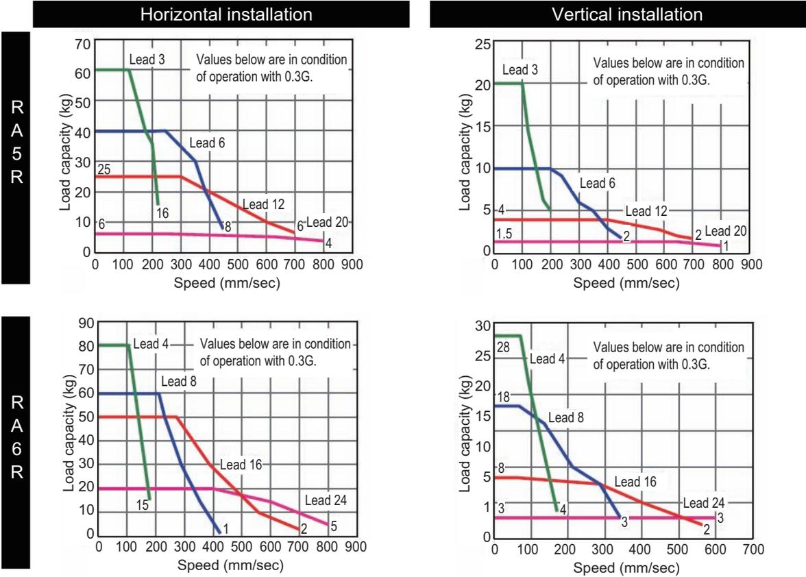
Correlation diagram of speed and loading capacity for the RCP4W rod type
