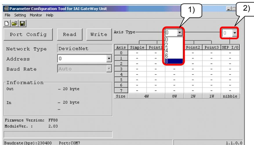
[Step 14] Once the setting of the number of axes is done, the cells for the operation mode settable to each axis turn to blank in response. For PIO Type and SEP I/O Mode, "\*" is displayed for a number equals to the number of set axis.
