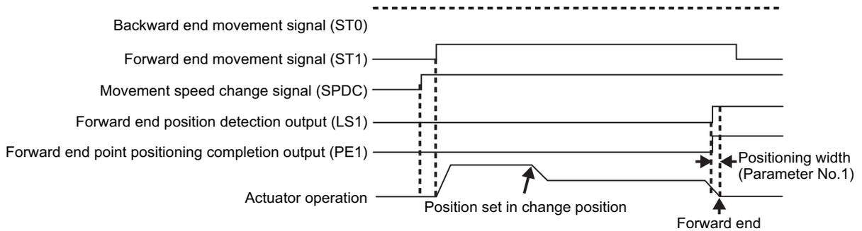
[11] Target Position Change = Operation Timing for Operation Patterns 2
