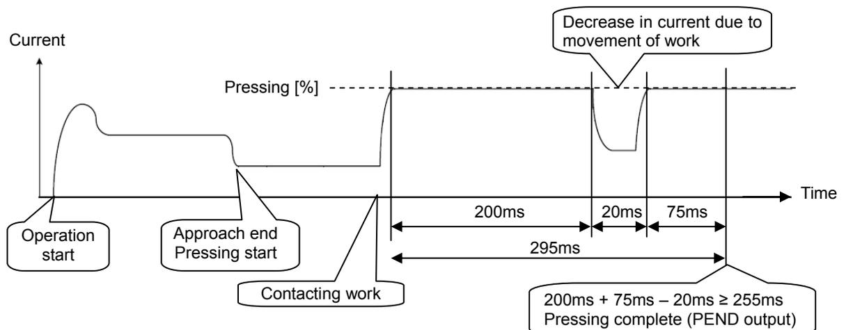
[9] Current limit value at stopping due to miss-pressing (Parameter No.9)
