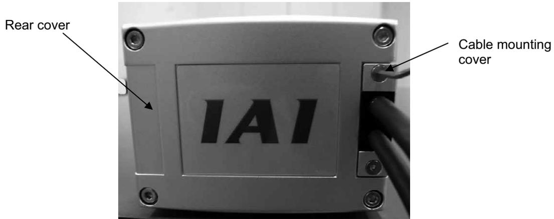
[2] Remove the four bolts used to secure the rear cover using an Allen wrench of 2.5 mm across flats for ISB and ISPB-SXM/SXL, or 3 mm across flats for all other models.
