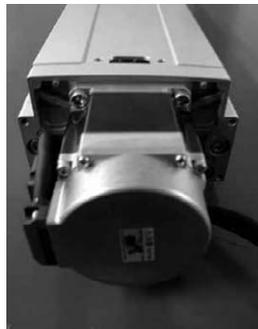
(6) Removing the motor unit
