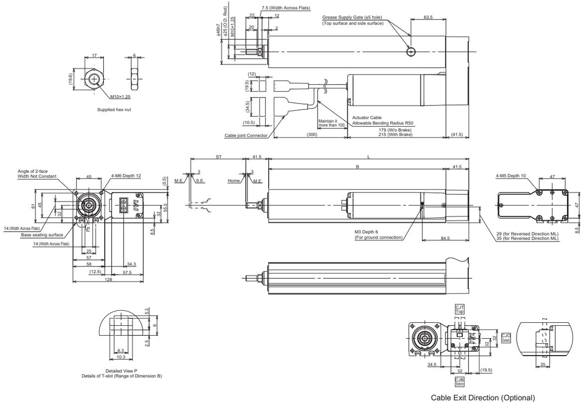
■ Dimensions and Mass by Stroke Unite: mm
