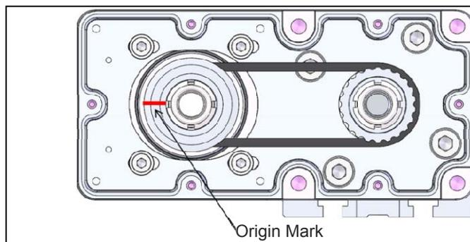
6) Apply tension in the force shown in the table below to the motor unit, and tighten the motor unit affixing screw in the tightening torque shown in the table below.
