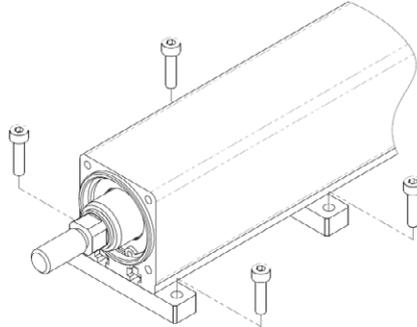
[Width direction pitch of foot bracket, attachment bolts and others]
