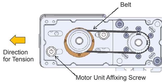
Tensile Force when Attaching Motor Unit
