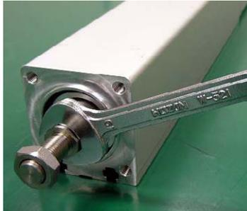
It cannot be used to apply a torque to the rod tip. Statically acceptable values and the rod tip maximum displacement angles (initial value reference) expected at that time are shown below. When the reaction force against the pressing operation is the side-way force, make sure it would not exceed the allowable load.
