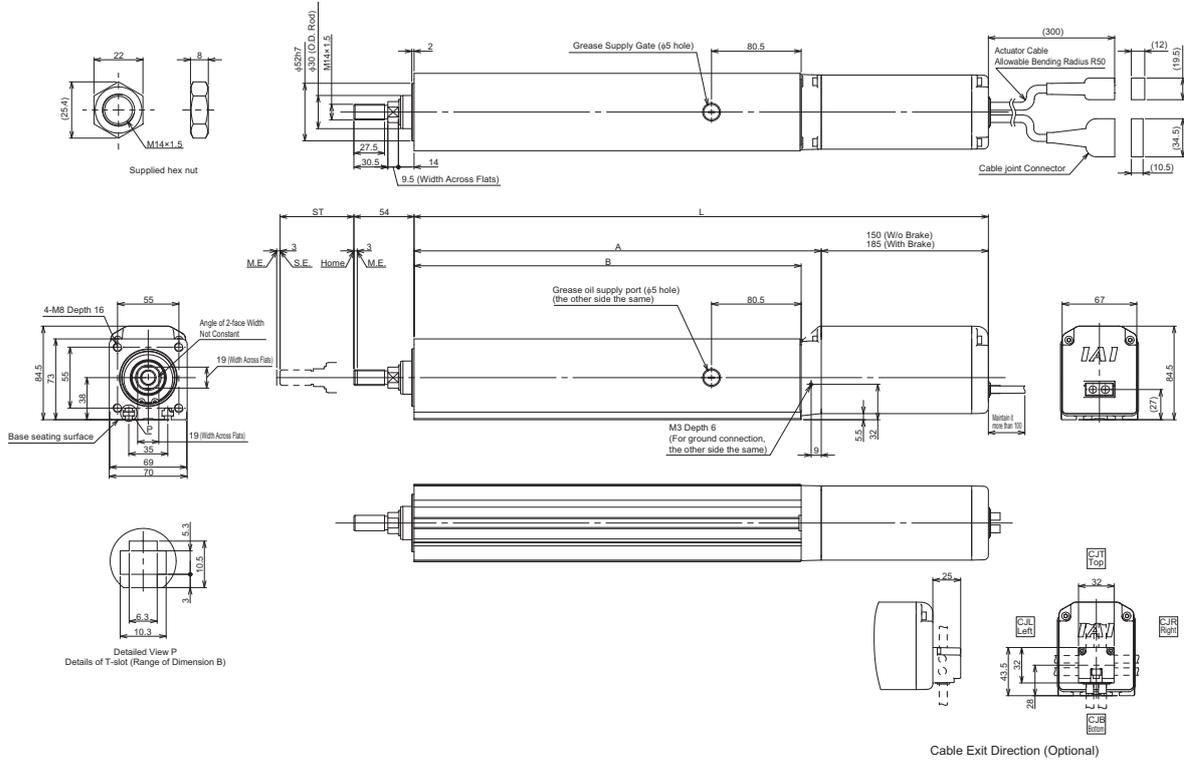
■ Dimensions and Mass by Stroke Unite: mm
