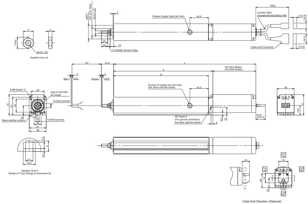
■ Dimensions and Mass by Stroke Unite: mm
