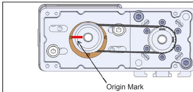
7) Apply tension in the force shown in the table below to the motor unit, and tighten the motor unit affixing screw in the tightening torque shown in the table below.
