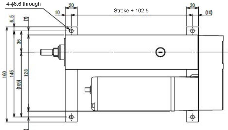
RCS4-RA6R Motor left reversed (ML) and Motor right reversed (MR)
