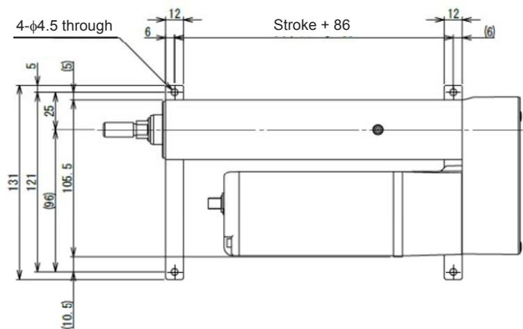
RCS4-RA4R Motor left reversed (ML) and Motor right reversed (MR)
