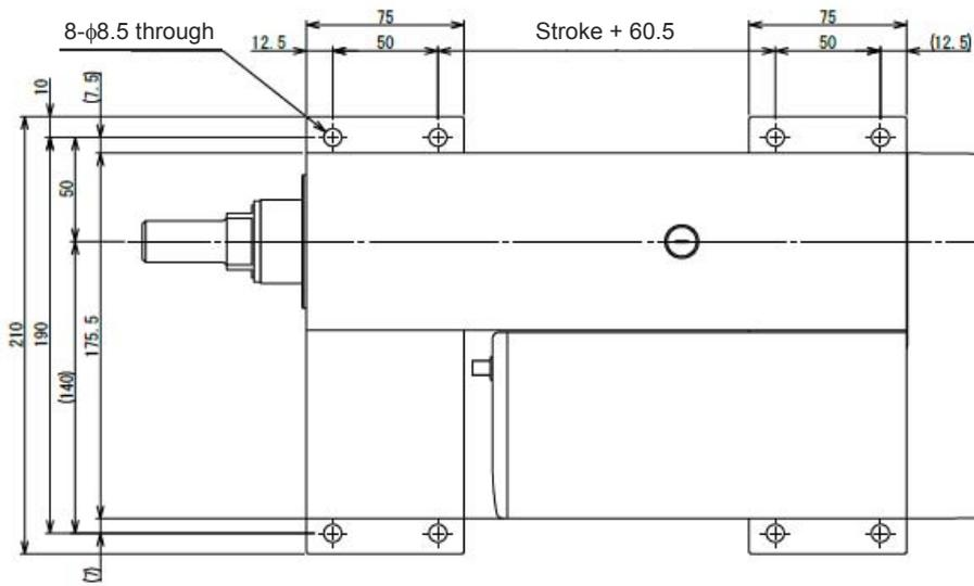
RCS4-RA8R Motor left reversed (ML) and Motor right reversed (MR)
