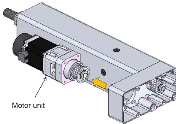
5) Attach the motor unit for replacement and hang the belt.
