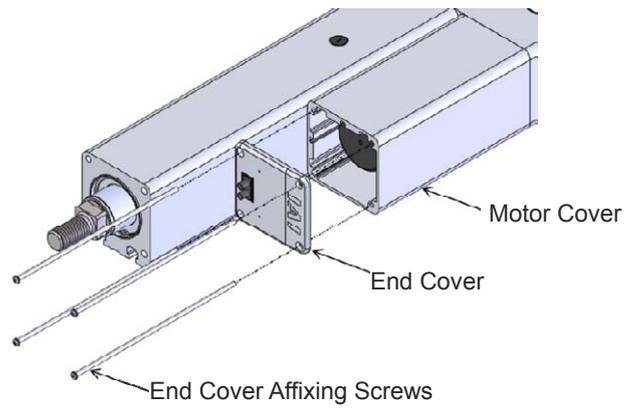
End Cover Affixing Screw Tightening Torque
