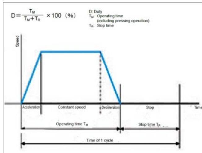
As the reference for duty available to use may differ depending on the operation conditions (payload, acceleration / deceleration, etc.), it is necessary to figure out the load factor LF and acceleration / deceleration time ratio  $t_{od}$  using the calculation formulae below and find it out from the graph.
