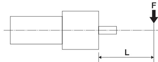
$$\text{Load Moment (N} \cdot \text{m)} = F \text{ (N)} \times L \text{ (m)}$$
