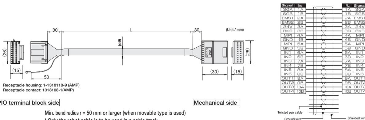
Min. bend radius  $r = 50$  mm or larger (when movable type is used)
