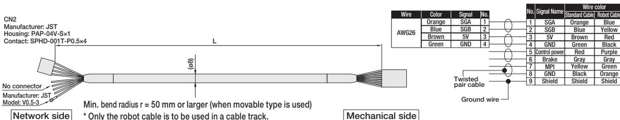
Min. bend radius  $r = 50$  mm or larger (when movable type is used)
