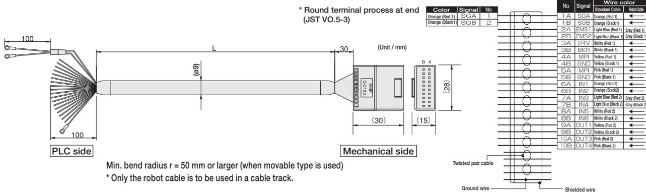
Min. bend radius  $r = 50$  mm or larger (when movable type is used)
