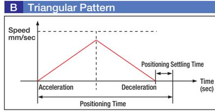
First confirm the movement pattern as trapezoidal or triangular, then calculate the positioning time using the respective equation.
