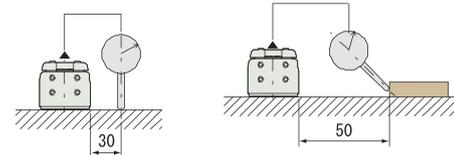
Condition: The above values were measured at 20°C. \*1: 0.05mm or less deviation from flatness.
