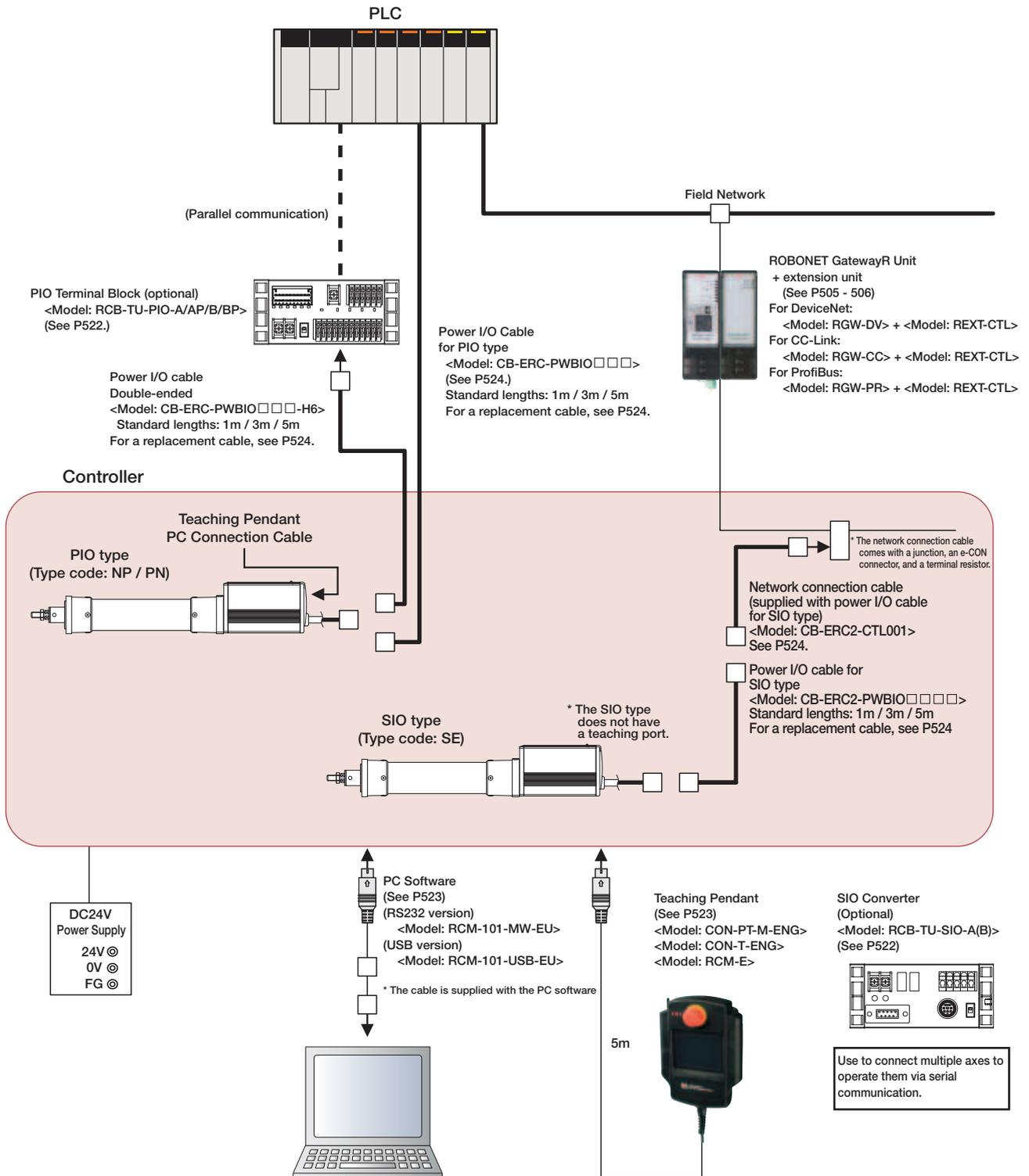
Wiring Diagram to Connect to a PC
