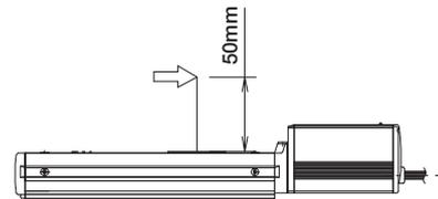
The SA7 rated moment is  $Ma = 13.8 \text{ (N}\cdot\text{m)}$  and  $13.8 \times 0.8 = 11.04 > 9.6$ , which means it is OK. Also, when pressing generates moment Mb, use the overhang calculation to similarly confirm that the moment is within 80% of the rated moment.
