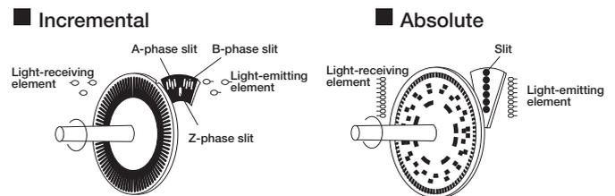
An incremental encoder detects the rotational angle and the RPM of the axis from the number of output pulses. To detect the rotational angle and the RPM, a counter is needed to cumulatively add the number of output pulses. An incremental encoder allows you to electrically increase the resolution by using the rise and fall points on the pulse waveform to double or quadruple the pulse generation frequency.
