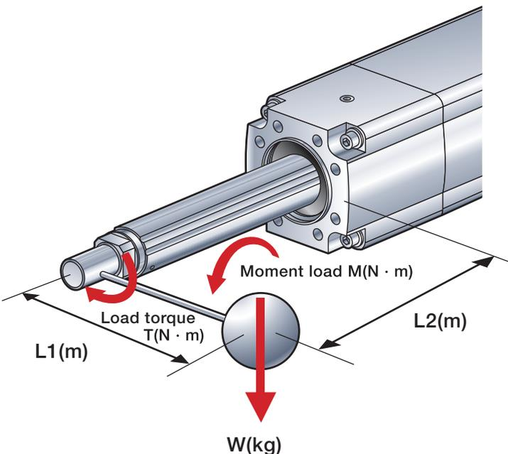
The ultra-high-thrust actuator can apply a load on the rod within the range of conditions calculated below.
