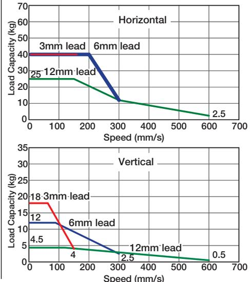
**Actuator Specifications** (Note 1) Please note that the maximum load capacity decreases as the speed increases.
