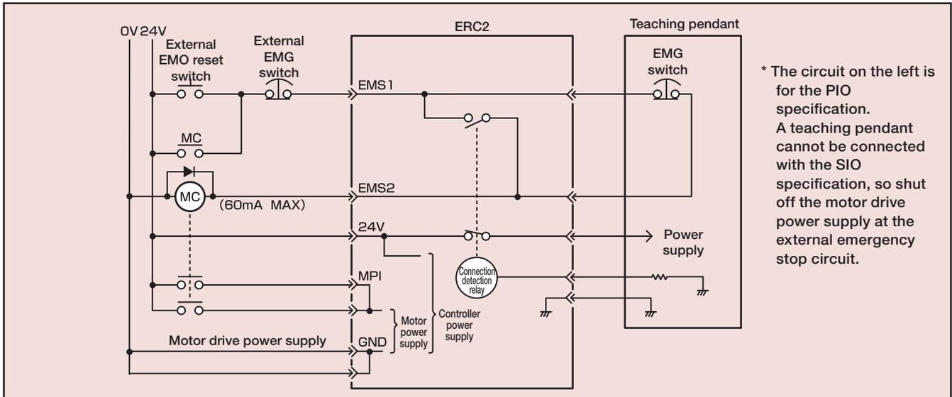
**Multiple Axis:** To provide an emergency stop circuit for a multiple-axes configuration, operate a relay using the EMG1 and EMG2 contacts of the SIO converter to cut off MPI (motor power) for each axis.
