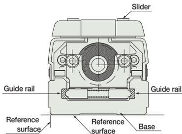
\* Parallelism does not apply to RCP2W-SA16C, due to its sliding guide.
