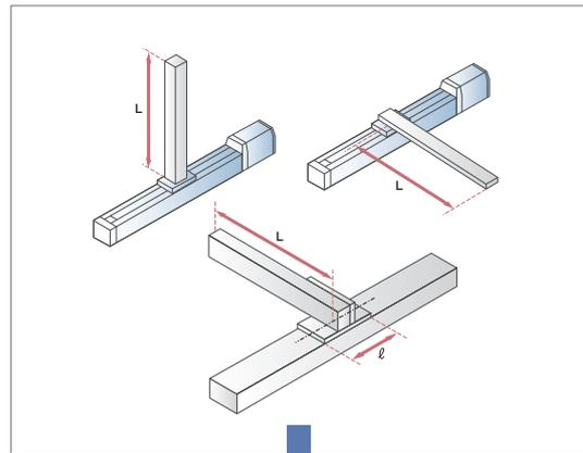
The allowable overhang load length is determined by the slider length.
