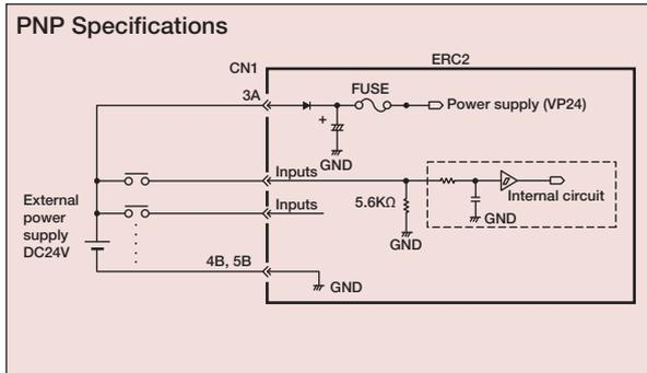
Output section External output specifications
