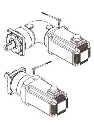
6 Install the plug, and the installinn complete.
