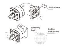
4 Please insert the motor shaft into the input shaft slowly to avoid impact, and make sure the surfaces of the motor flange and the reducer flange are stick together. Fasten the motor mounting bolt according to the specified fastening torque. (Refer to the Table 3)
