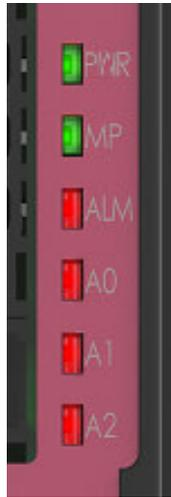
●PWR (Control power supply) / MP (Motor power supply)
