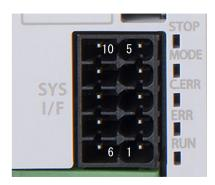
Cable connector name: DFMC1.5/5-ST-3.5 (Phoenix Contact)
