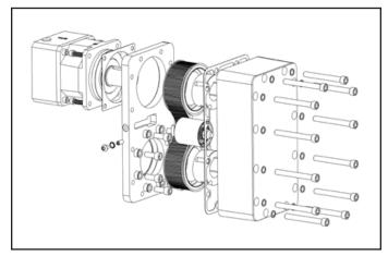
Figure 16 - Parallel Motor Mount Drive Train Assembly
