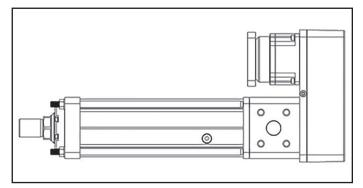
Figure 2 - FTX Actuator with Parallel Motor Mount
