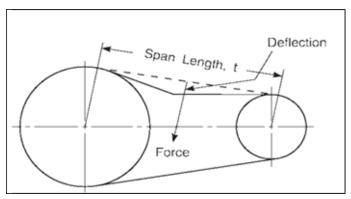
Figure 18 - Belt Tension Diagram
