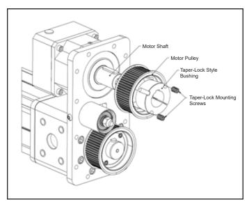
Figure 5 - Motor and Pulley with Taper-Lock Bushing
