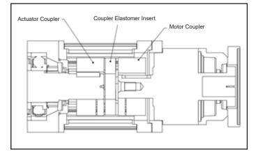
Figure 10 - Inline Mount Final Assembly
