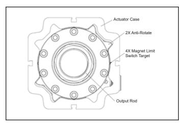
Figure 14 - Anti-Rotate Mechanism
