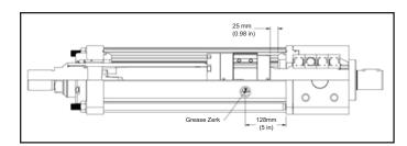
Figure 22 - Grease Port Location Apply grease into zerk through port in case, cycle actuator to distribute grease
