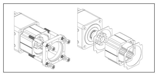
Figure 21 - Inline Housing Removal
