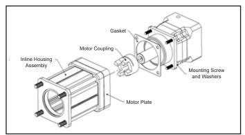
Figure 7 - Inline Motor Mounting
