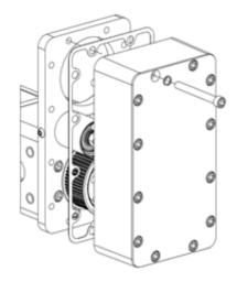
4. Remove screws from roller screw shaft pulley and use these same screws to push the pulley bushing off the pulley using the back out threads provided in the pulley or bushing. Then remove the motor pulley and bushing and remove the motor from the motor plate.
