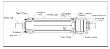
Figure 15 - Actuator Sealing Details
