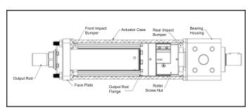
Figure 19 - Actuator End of Stroke Cushions
