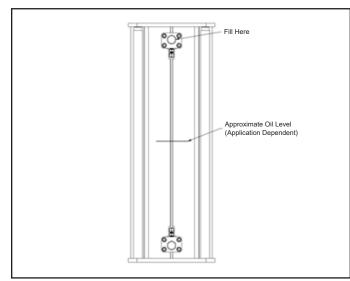
Figure 13 - Vertical Oil Fill Ports and Sight Tube
