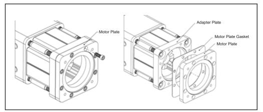
Figure 20 - Inline Mount Motor Plate Removal
