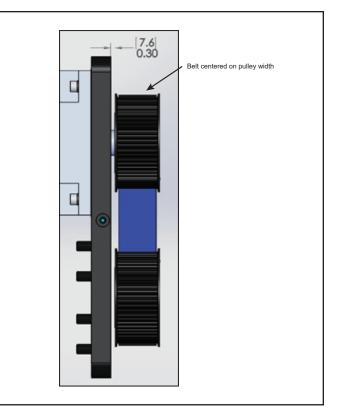
Figure 17 - Belt Distance from Motor Plate
