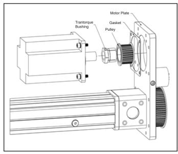
Figure 6 - Motor Pulley with keyless Style Bushing
