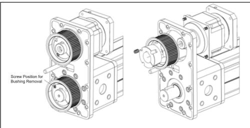
Figure 19 - Parallel Motor Mount Disassembly
