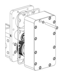
2. Attach motor or gearbox to motor plate using supplied mounting screws, washers and gasket.
