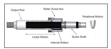
Figure 2 - Actuator Operating Principle
