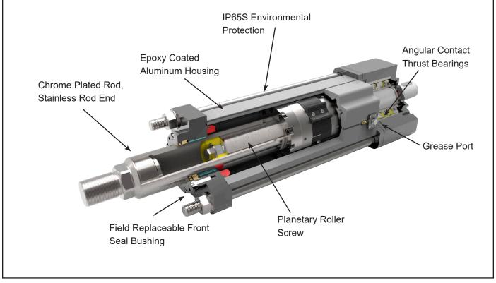
Figure 1 - FTX Series actuator features
