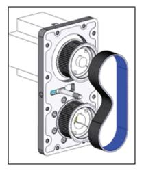
4. With the belt in place, the idler assembly can now be placed back over the T-bolt.
