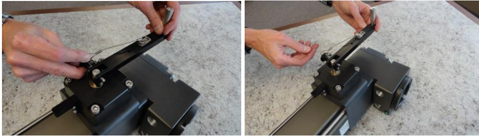
Re-insert Pin to Engage Hand Crank (Steps 4 & 5)
