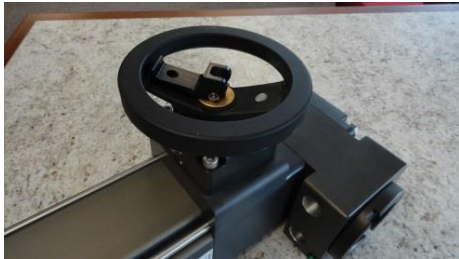
Handwheel in Engaged Position (Step 3)
