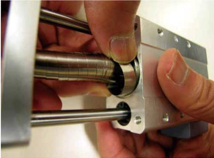
(2) Remove the spiral cover, telescoping it during removal.
