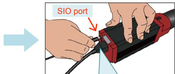
Insert the round connector with arrow mark downward
