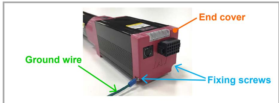
Use a tester to measure the continuity between the fixing screws and grounding surface to check whether it is grounded or not.
