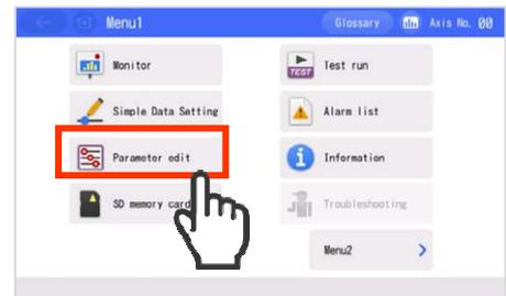
2 If the parameter edit password is set to a value other than "0000", enter the password and press the [ENT] key on the touch panel.
