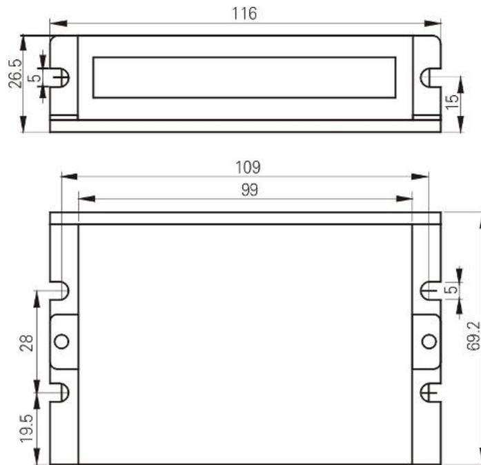
Figure 1: Mechanical specifications
