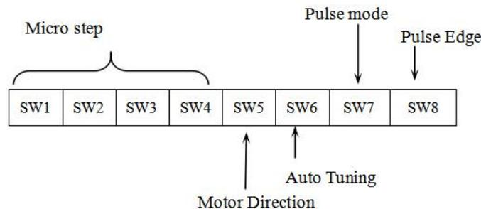
Figure 6 DIP switch Setting
