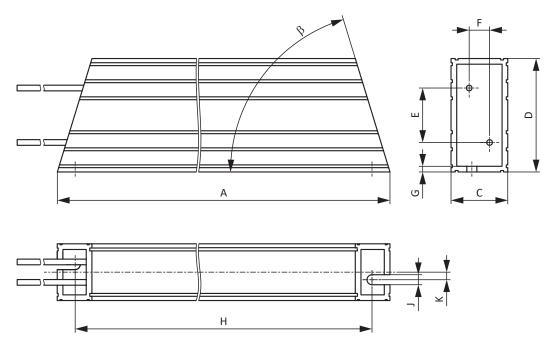
Fig. 7: GVADU, GBADU dimensional drawing
