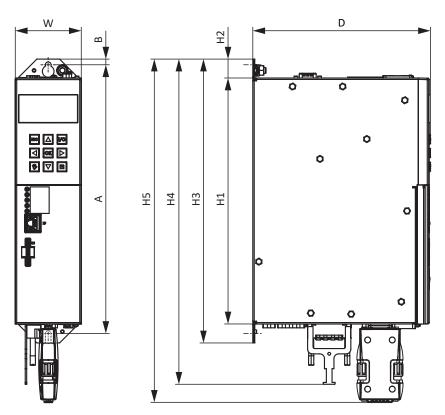
Fig. 5: SB6 dimensional drawing
