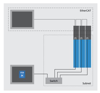
Fig. 76: Multi-axis scope: Network structure
