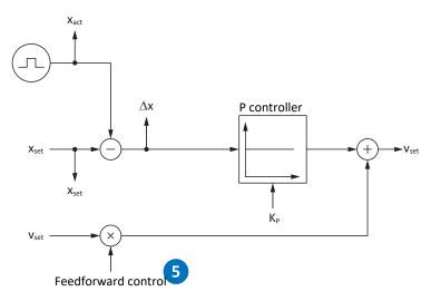
Fig. 49: Position controller – Feedforward control of the velocity controller
