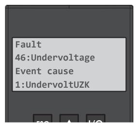
Fig. 66: Appearance of a fault on the display
