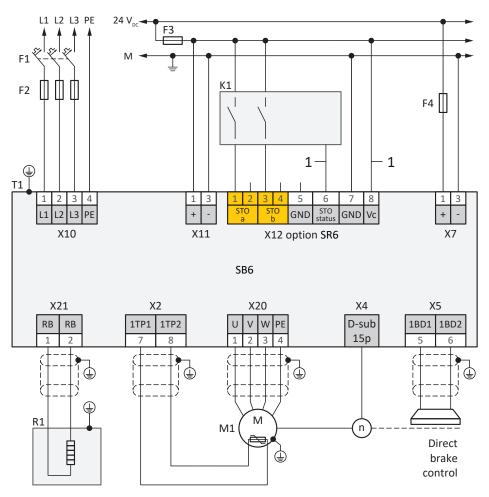
Fig. 77: Wiring example with direct brake control
