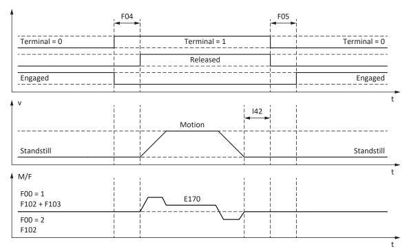
Fig. 58: Brake control for control mode B20 = 32: LM - sensorless vector control, 48: SSM-vector control incremental encoder, 64: SSM - vector control or 70: SLM - vector control
