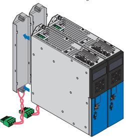
${\it 3.} \quad \hbox{Press the drive controller downward onto the guides.}$
