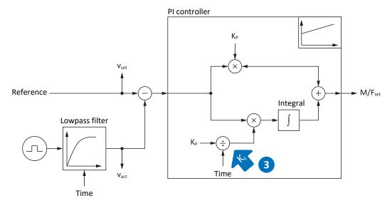
Fig. 46: Velocity controller – Integral coefficient
