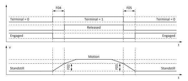
Fig. 55: Brake control for control mode B20 = 0: ASM - V/f-control or 1: ASM - V/f-slip compensated
