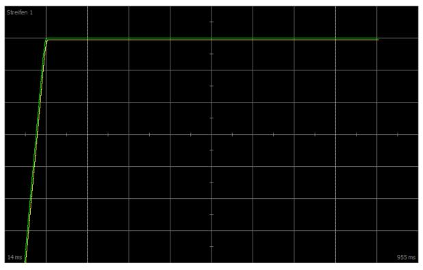
Fig. 44: Scope – Proportional coefficient of the velocity controller (C31), optimized value
