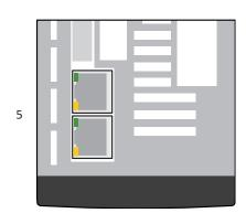
Fig. 64: Positions of the diagnostic LEDs on the front and top of the drive controller
