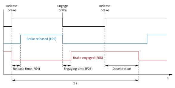
Fig. 59: Minimum time between 2 release processes for the brake
