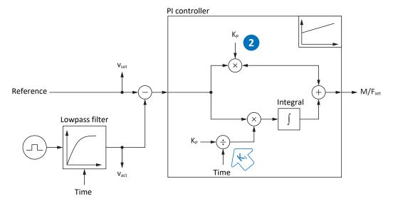
Fig. 41: Velocity controller – Proportional coefficient
