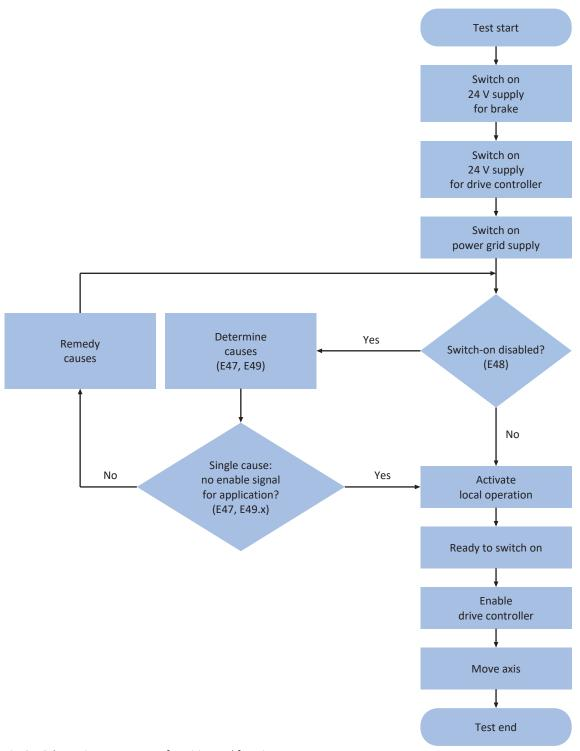
Fig. 37: Schematic test sequence for wiring and function test
