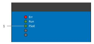
Fig. 68: LED for the FSoE state
