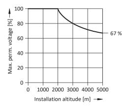
Fig. 14: Derating the voltage depending on installation elevation
