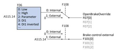
Fig. 53: Brake control in CiA 402 applications
