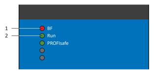
Fig. 69: LEDs for the PROFINET state
