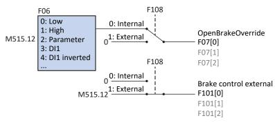
Fig. 54: Brake control in PROFIdrive applications
