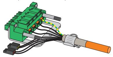
4. Attach terminal X20 and tighten the screws of X20. After tightening the screws, make sure that there is sufficient distance between the cores and terminal X20.
