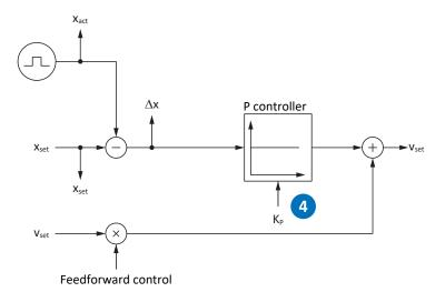
Fig. 48: Position controller – Proportional coefficient
