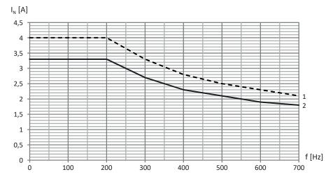
Fig. 9: Derating the nominal current depending on the clock frequency, TEP3720-0ES41
