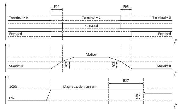
Fig. 57: Brake control for control mode B20 = 3: ASM - sensorless vector control
