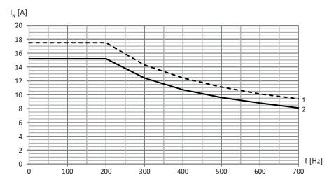
Fig. 10: Derating the nominal current depending on the clock frequency, TEP3820-0CS41
