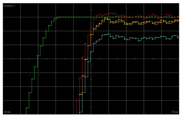
Fig. 47: Scope - Integral coefficient of the velocity controller (C32)
