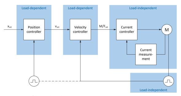
Fig. 38: Structure of the control cascade
