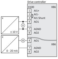
Fig. 28: X100: Actuator connection example
