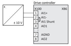
Fig. 27: X100: Sensor connection example 2
