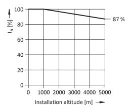
Fig. 13: Derating the nominal current depending on installation elevation
