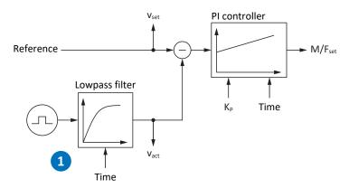
Fig. 40: Velocity controller – Filters for the actual velocity
