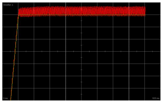
Fig. 43: Scope – Proportional coefficient of the velocity controller (C31), continuous oscillations
