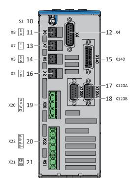
Fig. 23: SB6 connection overview, top and bottom of device
