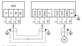
Fig. 31: TEP output choke connection example
