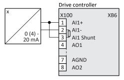
Fig. 26: X100: Sensor connection example 1
