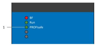
Fig. 70: LED for the PROFIsafe state
