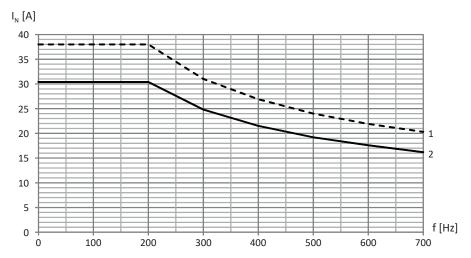
Fig. 11: Derating the nominal current depending on the clock frequency, TEP4020-0RS41
