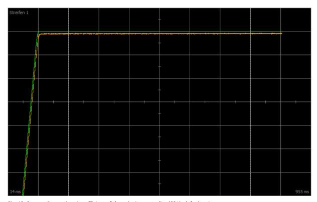
Fig. 42: Scope – Proportional coefficient of the velocity controller (C31), default value
