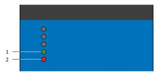
Fig. 65: LEDs for the state of the drive controller
