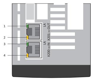
Fig. 72: LEDs for the state of the EtherCAT network connection
