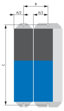
Fig. 17: SB6 drilling diagram
