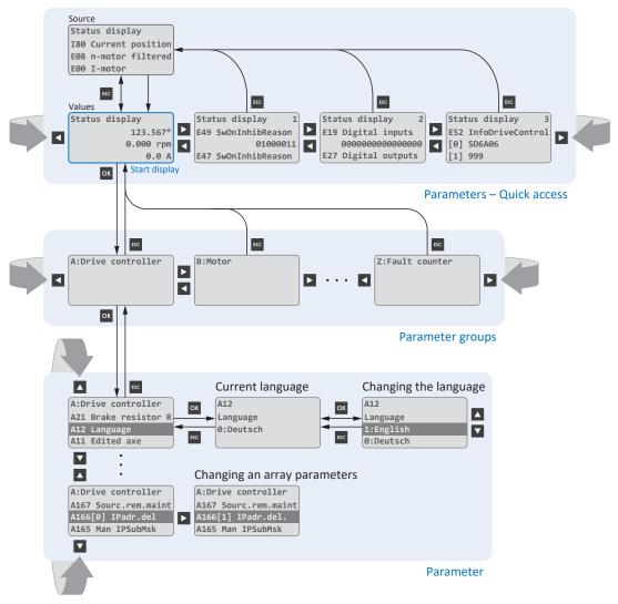
Fig. 35: Menu structure and navigation using the optional OP6 operating unit
