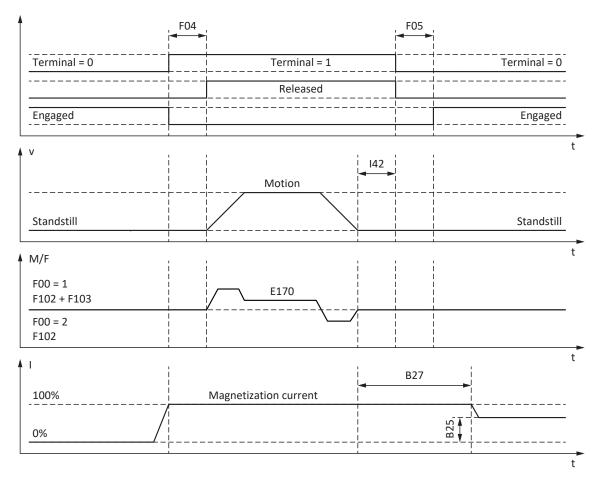
Fig. 56: Brake control for control mode B20 = 2: ASM - vector control
