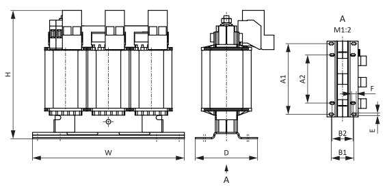
Fig. 8: TEP dimensional drawing
