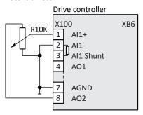
Fig. 25: X100: Potentiometer connection example
