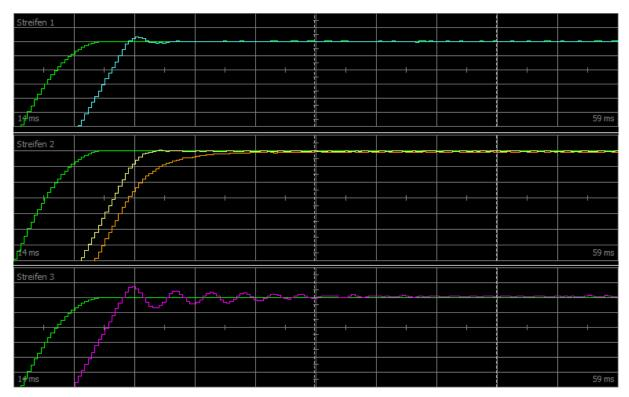
Fig. 45: Scope – Proportional coefficient of the velocity controller (C31), overshooting
