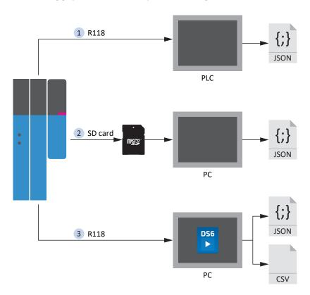
Fig. 63: Predictive Maintenance: Options for readout
