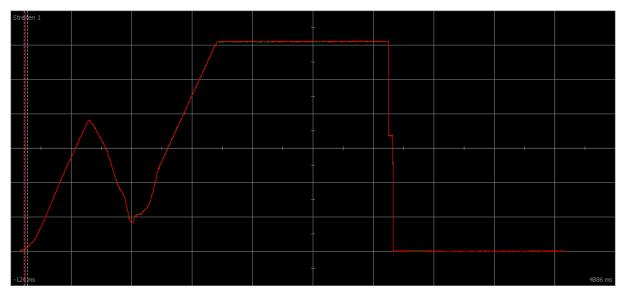
Fig. 51: Scope – Motor reaches saturation with tracking (B59)
