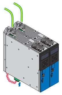
⇒ The installation is completed. In the next step, connect the drive controller.
