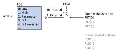
Fig. 52: Brake control in Drive Based applications
