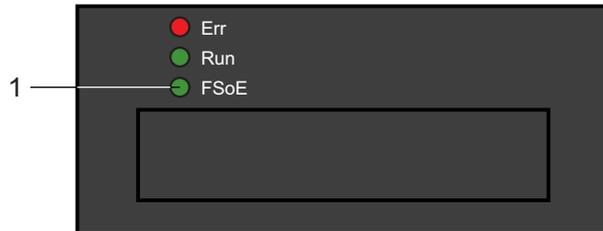
Fig. 8: FSoE LED on the front of the drive controller
