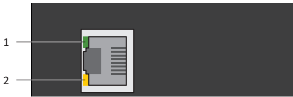
Fig. 93: LEDs for the state of the service network connection
