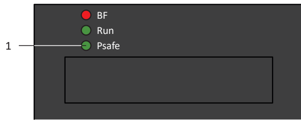
Fig. 92: LED for the PROFIsafe state
