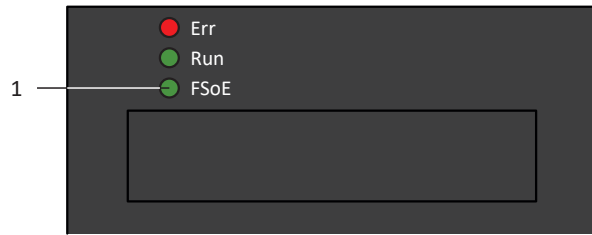
Fig. 90: LED for the FSoE state
