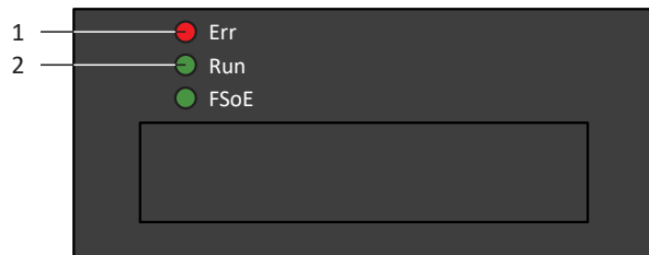
Fig. 88: LEDs for the EtherCAT state
