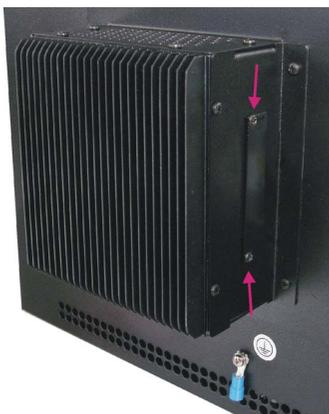
Push the metal plate to the side. The following graphic shows the opened housing of the MC6 of type MC6x10 and MC6x11 as well as the slot of the memory card.
