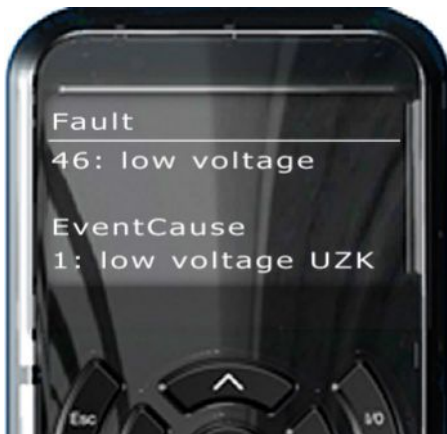
Fig. 97: Appearance of a fault on the display
